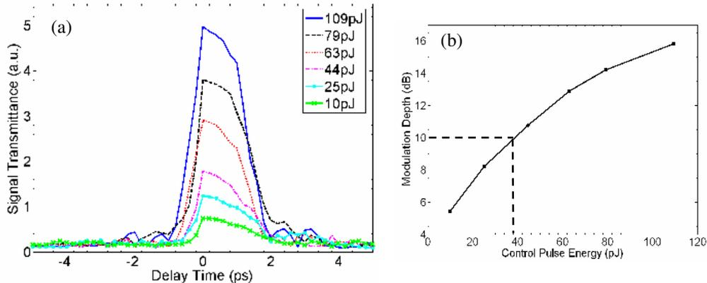
Fig. 3. (a). Transmittance of the signal pulses through a 3- $\mu\text{m}$ -wide, 1-mm-long waveguide versus signal-control delay time, for different values of the control pulse energy. (b) Signal modulation depth (i.e. maximum control-pulse-induced increase in the signal transmittance relative to the fully non-saturated case) versus control pulse energy, as determined from the traces of (a).
