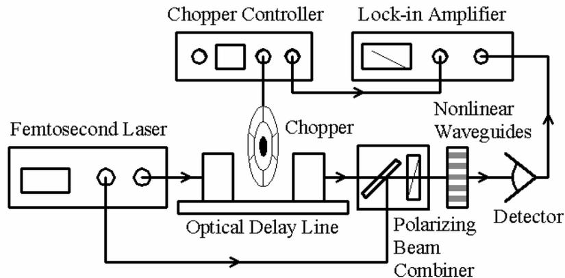
Fig. 2. Pump-probe measurement setup used in this work.
