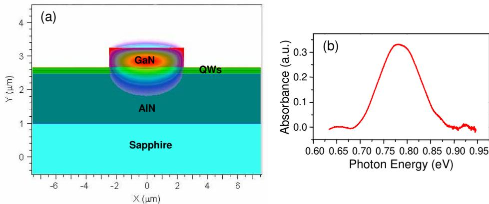
Fig. 1. (a). Schematic cross-section of the GaN/AlN waveguide structure used in this work, and color map of the intensity profile of its fundamental TM mode at  $1.55 \mu\text{m}$  (computed using commercial software based on the beam propagation method [16]). The refractive index values used in this simulation are 1.746 for sapphire, 2.335 for GaN, and 2.031 for AlN [17]. (b) Measured ISB absorption spectrum of the QW active material.
