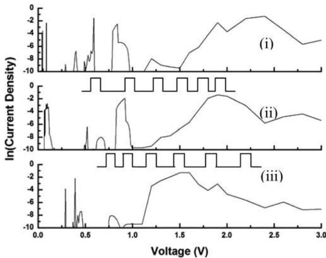
FIG. 5. Current density vs voltage for MQW structure (number of wells = 5) with (i) uniform structure (barrier width = 2.4 nm, well width = 6 nm, and barrier height = 0.5 eV), (ii) well width decreasing toward the right (values = 6, 5.5, 5, 4.5, and 4 nm), (iii) well widths increasing toward the right side (values = 3, 4, 5, 6, and 7 nm). In each case, the barrier width is fixed (2.4 nm) and the barrier height is fixed (0.5 eV).
