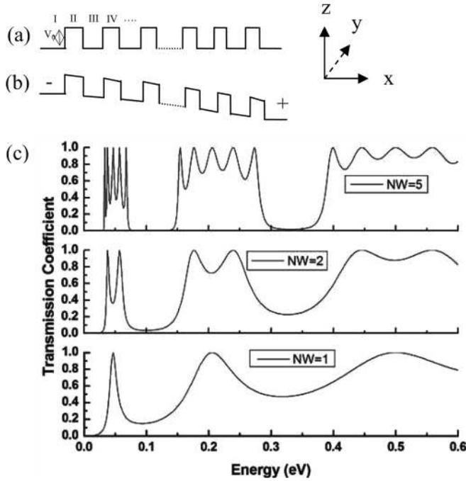
FIG. 1. (a) Conduction band (CB) diagram of an unbiased uniform MQW structure (e.g.,  $\text{Al}_{0.5}\text{Ga}_{0.5}\text{As}/\text{GaAs}$  has a CB offset of 0.5 eV), (b) biased MQW structure, (c) transmission coefficient vs energy of the uniform MQW structure with the number of wells (NW) as a parameter. The barrier width is fixed (0.8 nm), the well width is fixed (8 nm), and the barrier height is fixed (0.5 eV).
