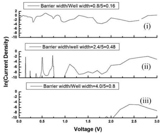
FIG. 3. Current density vs voltage plot of uniform MQW structure (number of wells = 5) with the barrier-to-well width (B/W) ratio (i) 0.16, (ii) 0.48, and (iii) 0.8. The well width is fixed (5 nm) and the barrier height is fixed (0.5 eV).
