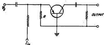
FIG. 1. The basic grounded base transistor amplifier for use as multiplier.
