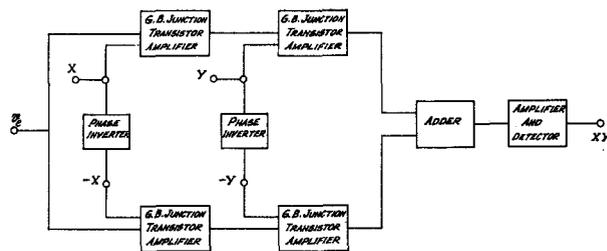
FIG. 3. Schematic diagram of the four-quadrant transistorized multiplier.
