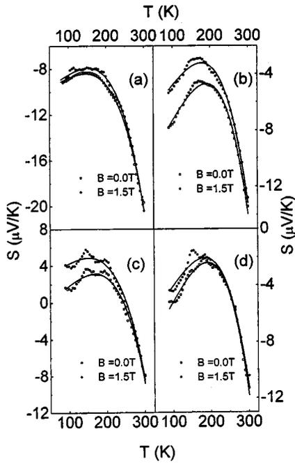
FIG. 4. Temperature and magnetic-field dependent Seebeck coefficient ( $S$ ) of four different samples with (a)  $y=0.05$ , (b) 0.1, (c) 0.15, and (d) 0.3. Solid lines are best-fit lines to the Eq. (4).
