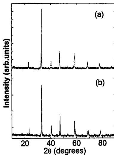
FIG. 1. XRD pattern of the two samples with (a)  $y=0.0$  and (b)  $y=0.15$  showing single-phase perovskite structure.
