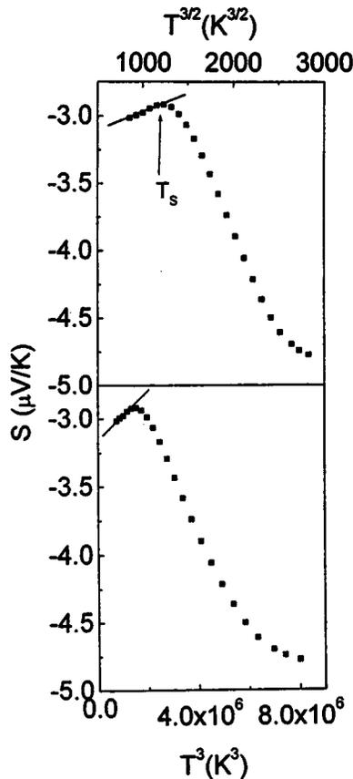
FIG. 6.  $S$  vs  $T^{1.5}$  and  $S$  vs  $T^3$  plot for the sample  $\text{La}_{0.7}\text{Ca}_{0.3}\text{MnO}_3$ . An almost linear variation of  $S$  with  $T^{1.5}$  and  $T^3$  below  $T_S$  suggest the presence of both phonon and magnon drag effects in the low-temperature region.
