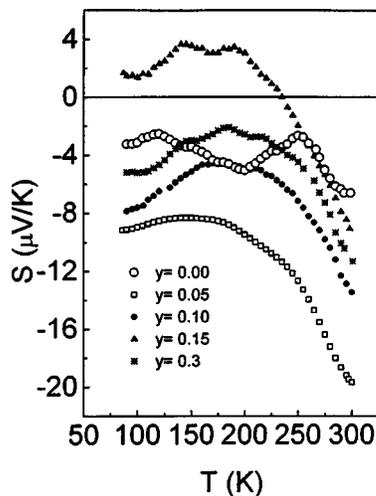
FIG. 3. Thermal variation of Seebeck coefficient ( $S$ ) of  $\text{La}_{0.7}\text{Ca}_{0.3-y}\text{Na}_y\text{MnO}_3$  with  $y=0, 0.05, 0.1, 0.15,$  and  $0.3$  without applying magnetic field.
