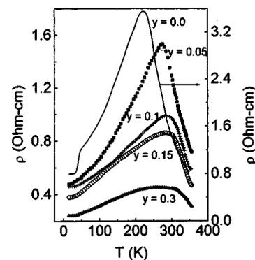
FIG. 2. Thermal variation of resistivity ( $\rho$ ) of  $\text{La}_{0.7}\text{Ca}_{0.3-y}\text{Na}_y\text{MnO}_3$  with  $y=0, 0.05, 0.1, 0.15$ , and  $0.3$ .
