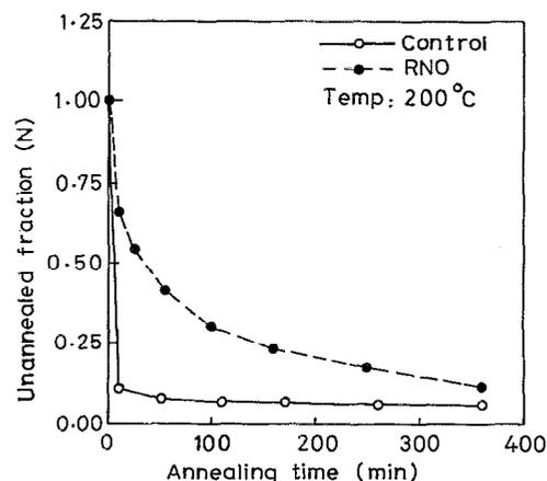
FIG. 4. Isothermal detrapping of the radiation-induced trapped charges in control oxide as well as RNO devices.
