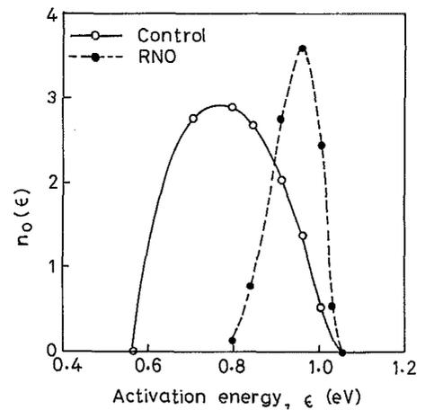
FIG. 6. Activation energy distribution of annealing of the radiation-induced trapped charges in control oxide as well as RNO devices.
