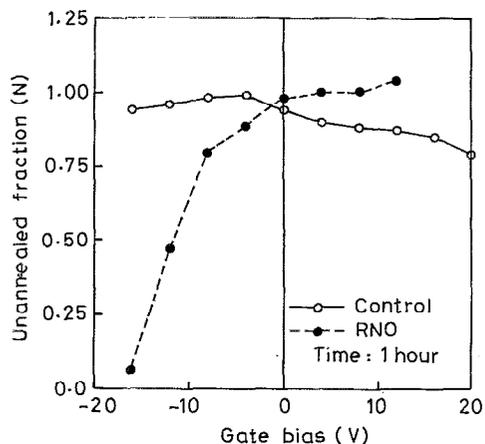
FIG. 1. Field detrapping of the radiation-induced trapped charges in control oxide as well as RNO devices at different gate bias conditions.
