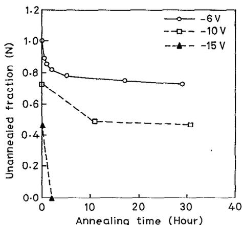
FIG. 2. Field detrapping of the radiation-induced trapped charges in RNO devices as a function of time.
