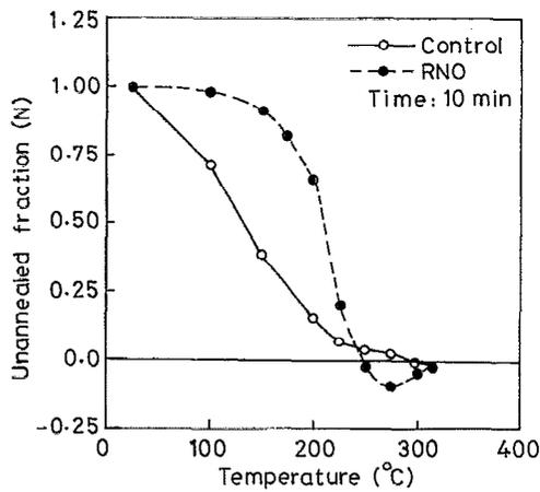
FIG. 5. Isochronal detrapping of the radiation-induced trapped charges in control oxide as well as RNO devices.
