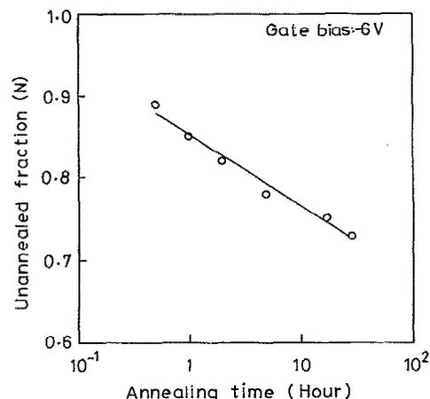
FIG. 3. Field detrapping of the radiation-induced trapped charges in RNO devices.
