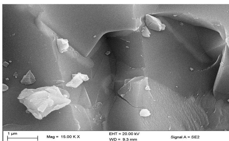
**Figure 2.** SEM Micrograph analysis of  $\text{Cr}_2\text{O}_3$  doped L1 samples heated at 1600°C.
