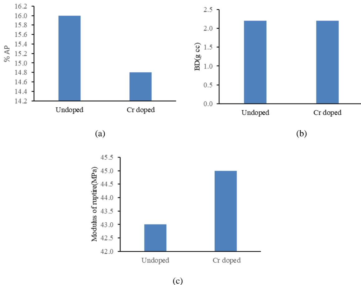
**Figure 1.** Variation in (a) AP, (b) BD, and (c) MOR of sintered  $\text{Cr}_2\text{O}_3$  doped samples at  $1600^\circ\text{C}$  temperature
