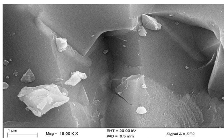
**Figure 6.** SEM Micrograph analysis of MgO doped L3 samples heated at 1600°C
