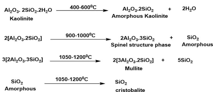
**Scheme 1.** Phase transformation during heating of kaolinitic clay [11].
