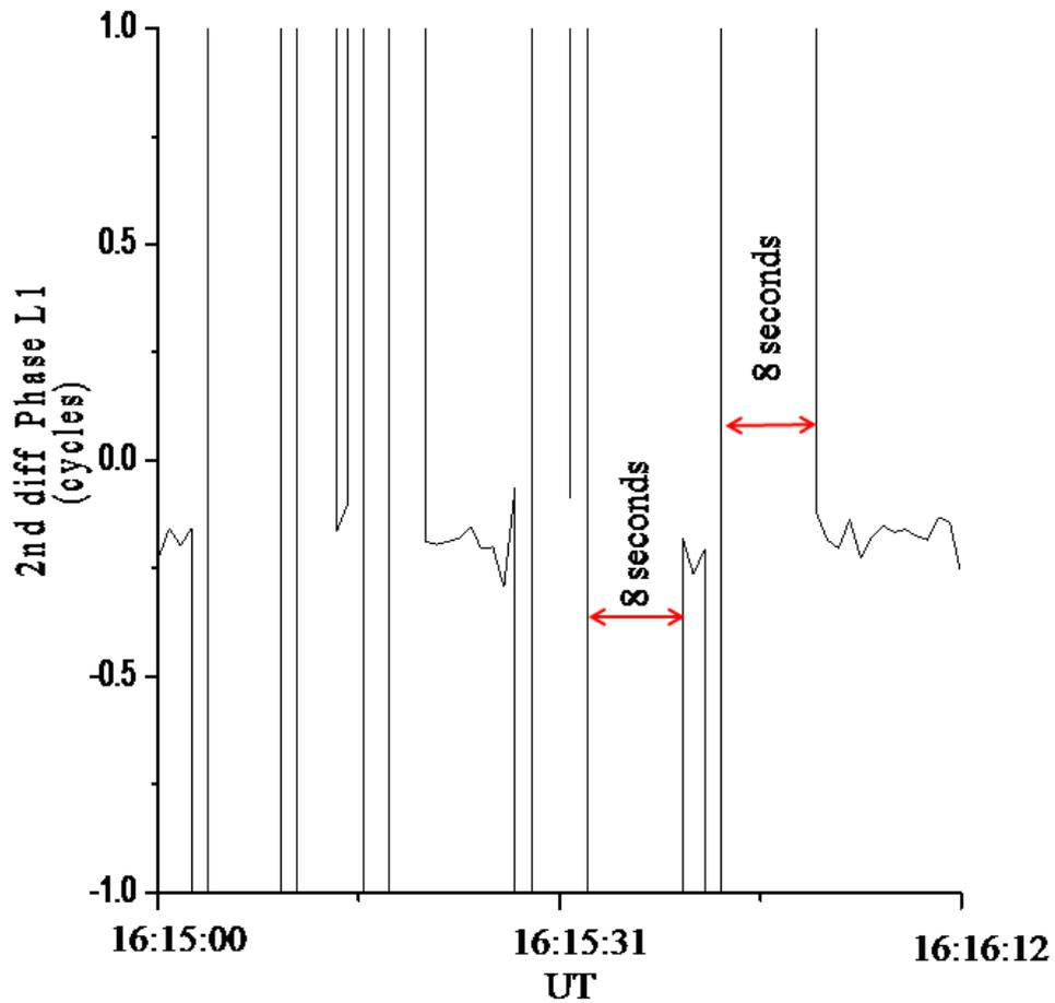
Figure 5: Second difference of the recorded phase on the GPS SV10 L1 signal over a brief interval 16:15-16:16UT to show occurrence of cycle slips. Discontinuities in phase of duration 8s could be found after 16:15:31UT on the SV10 link indicating occurrence of cycle slips
