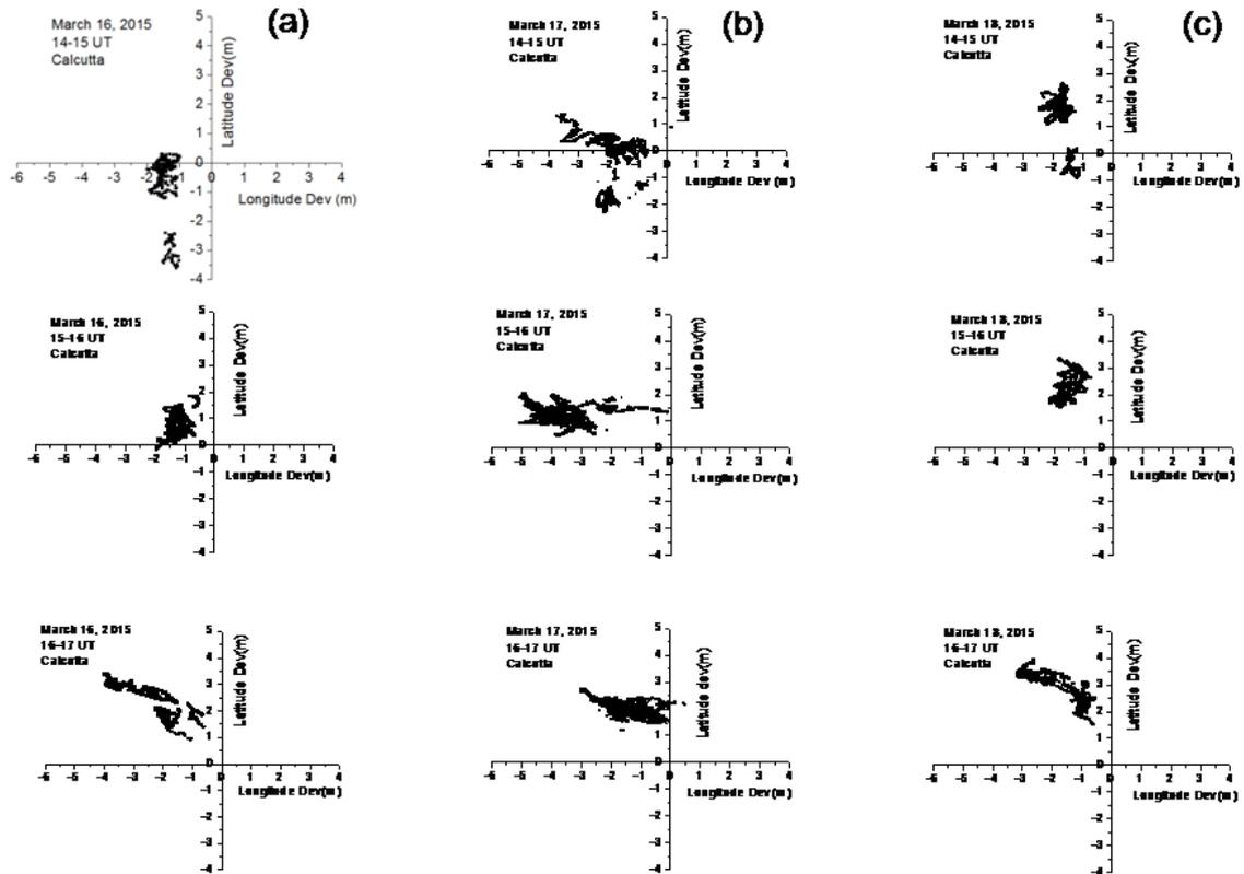
Figure 8: Position deviations of the receiver measured at Calcutta, for each hour of 14:00-17:00UT of March 16, 17 and 18, 2015. The position deviations, expressed in terms of latitude and longitude in meters, have been calculated taking the reference at 00:00UT
