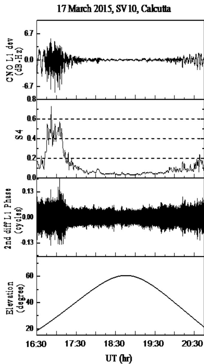
Figure 4: CNO deviations for scintillations observed from Calcutta on SV10, S4, second difference of phase and satellite elevation angle variations during 16:30-20:45UT of March 17, 2015
