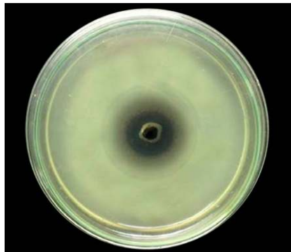
Figure 13 Antibacterial activity of Ag NPs assayed by the agar diffusion method in petri plate. Ag NPs, poured in the circular well, showed the zone of inhibition against Bacillus subtilis . The cavity of the petri plate was filled with Ag NPs solution (0.2 mg/ml).
