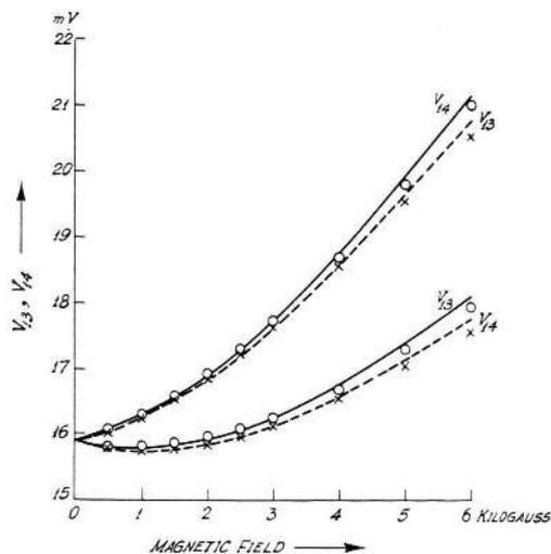
Fig. 2. Showing the variation of  $V_{13}$  and  $V_{14}$  with magnetic field (broken line for direct and continuous line for reverse field). Crosses and hollow circles show experimental points for direct and reverse magnetic fields respectively.
