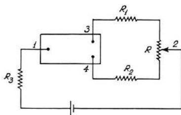
Fig. 1. Schematic diagram of the 3-terminal device.
