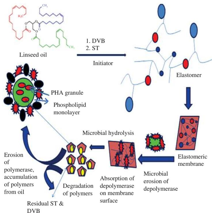
**Figure 6** Schematic of the microbial degradation of the elastomers and the formation of a new polymer.
