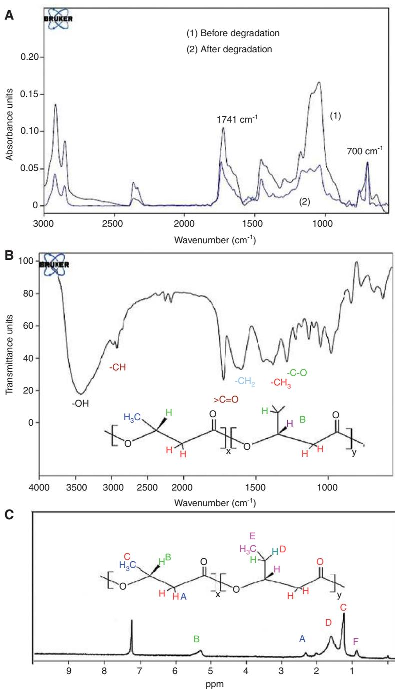
**Figure 8** (A) FTIR spectra of S8Lin65 before and after degradation. (B) FTIR spectrum of the produced polymer as cell mass. (C)  $^1\text{H NMR}$  spectrum of the produced polymer as cell mass.
