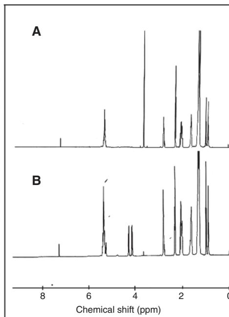
**Figure 4**  $^1\text{H}$  NMR spectra of (A) the methyl ester of linseed oil and (B) linseed oil.
