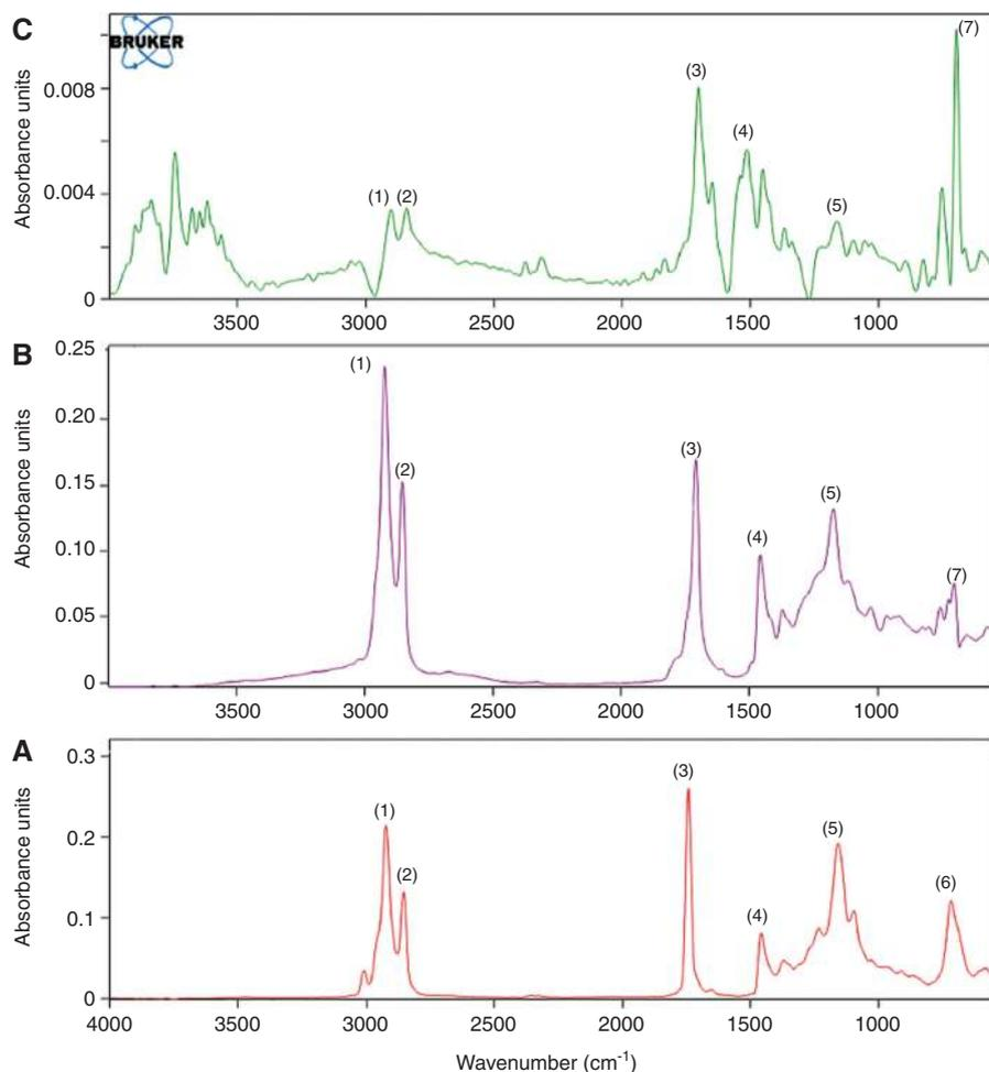
**Figure 2** FTIR spectra of (A) linseed oil, (B) soluble extract of S5Lin50, and (C) insoluble extract of S5Lin50.
