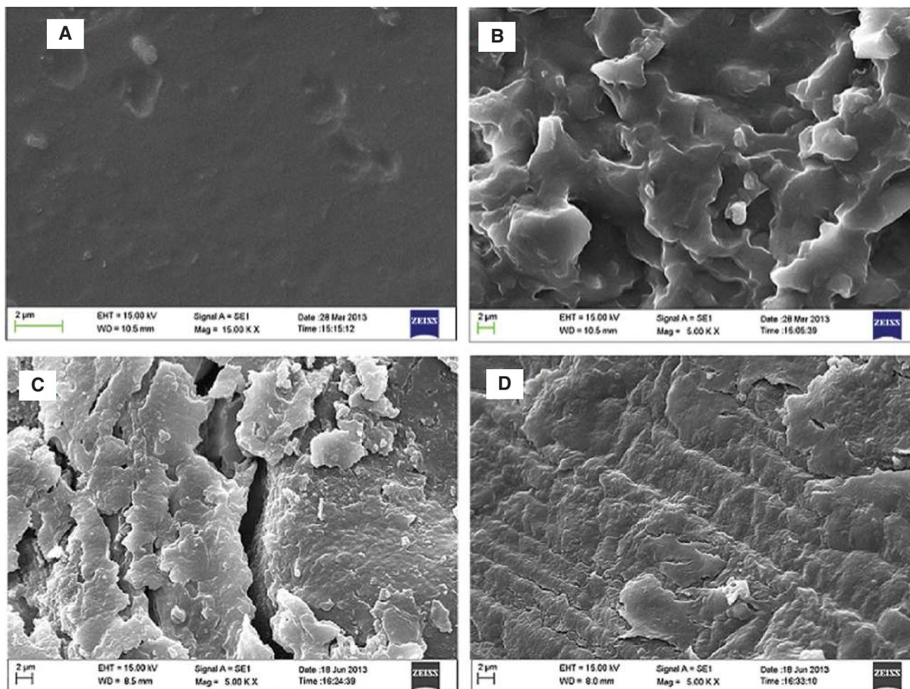
**Figure 9** Scanning electron micrographs of (A) S8Lin65 before degradation, (B) S8Lin65 after degradation, (C) S7Lin60 after degradation, and (D) S5Lin50 after degradation.
