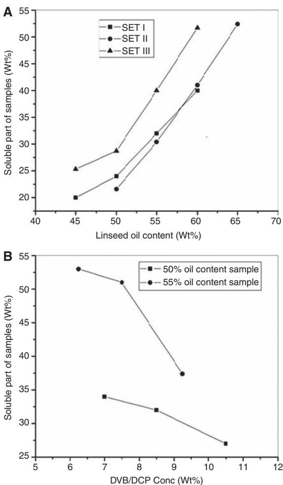
**Figure 1** Soxhlet extraction results of different elastomers of (A) SET I, SET II, and SET III, and (B) SET IV.
