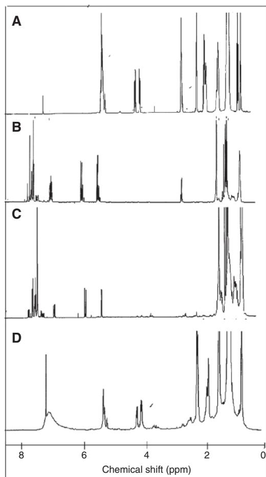
**Figure 5**  $^1\text{H}$  NMR spectra of (A) linseed oil, (B) styrene, (C) divinylbenzene, and (D) the soluble extract of S2Lin40 (Oil50+ST25+17DVB+In8).
