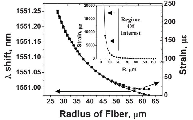
FIG. 2. Comparison of theoretical and experimental values of strain (in terms of wavelength shift) as a function of radius of the grating fiber. The inset is extended theoretical plot of strain as a function of radius of the fiber,  $\Delta\varepsilon \propto 1/\pi r^2$ .
