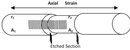
FIG. 1. Schematic diagram of the partially etched FBG sensor under longitudinal strain.  $(r_1, A_1)$  and  $(r_2, A_2)$  denote radius and area of cross sections of nonetched grating (FBG-1) and etched grating (FBG-2) fiber, respectively.
