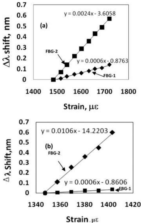
FIG. 4. Plots (a) and (b) compare wavelength shift for FBG-1 with the shift in FBG-2 of diameter 61.75 and  $32 \mu\text{m}$ , respectively, as a function of strain.
