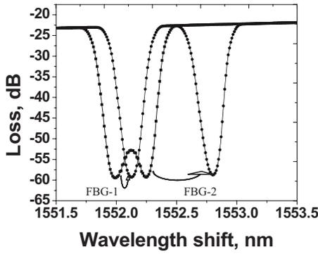
FIG. 3. Shift of two peaks under arbitrary tension. The peak for etched FBG-2 experiences approximately four times shift compared to nonetched FBG-1.
