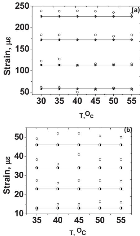
FIG. 5. Comparison between applied and measured strains by the proposed model. The half-filled circle points on solid lines are applied strain at different temperature. The empty circle point nearest to the half-filled circle point is the respective strain obtained from the model.
