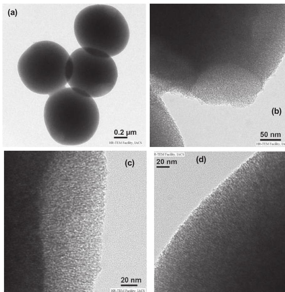
**Fig. 4.** HRTEM images of SMSNP-BA (Panel a, b, c) and SMSNP (Panel d).
