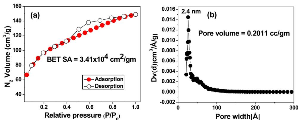
**Fig. 3.** N<sub>2</sub> adsorption isotherm and pore size distribution of SMSNP-BA. Adsorption points are marked by filled circle whereas those for desorption are marked by empty circles.
