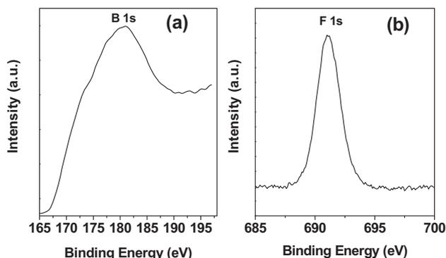
Fig. 2. XPS profile of B1s (a) and F1s (b) of SMSNP-BA.
