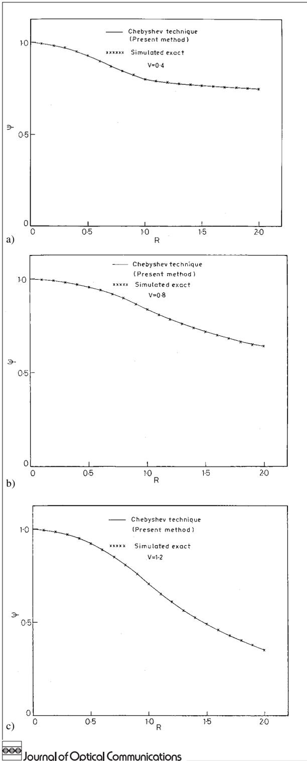
Fig. 1: Variation of normalised field  $\psi$  with normalised radius  $R$  for single-mode step index fiber having (a)  $V = 0.4$ , (b)  $V = 0.8$  and (c)  $V = 1.2$
