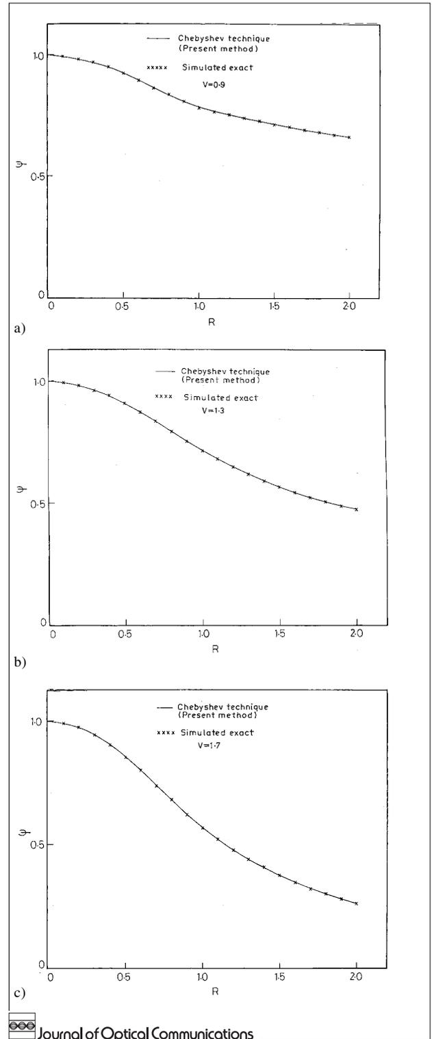
Fig. 2: Variation of normalised field  $\psi$  with normalised radius  $R$  for single-mode parabolic index fiber having (a)  $V = 0.9$ , (b)  $V = 1.3$  and (c)  $V = 1.7$
