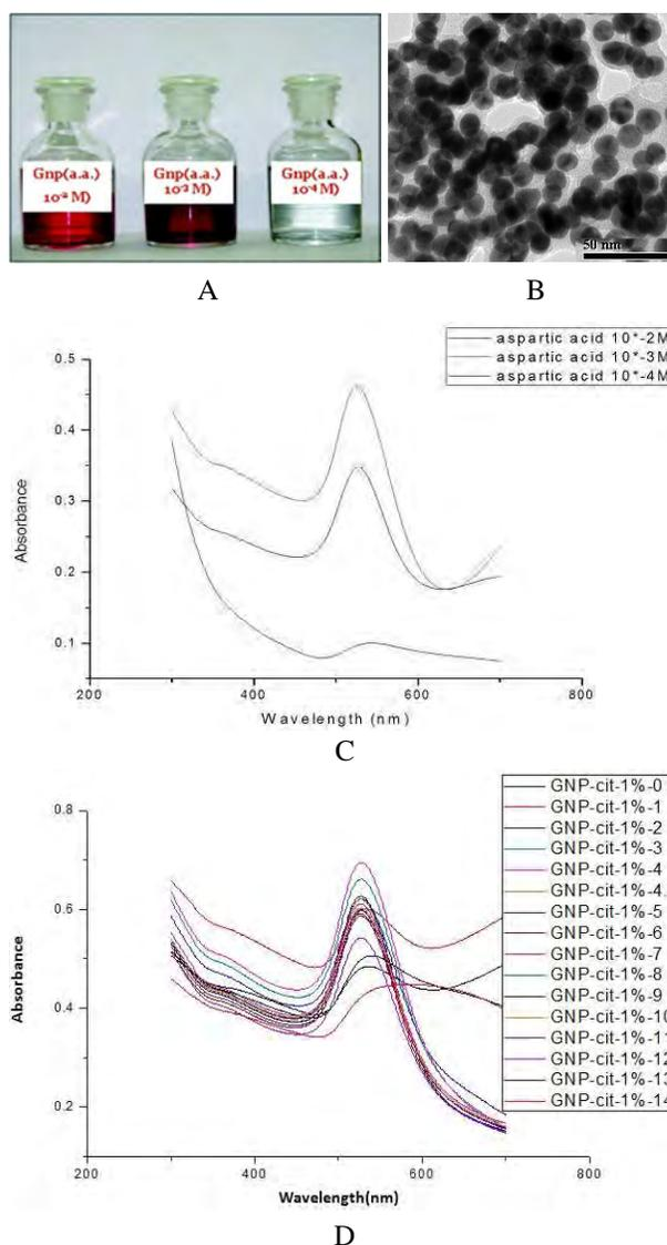
**Fig. 7:** A: Interface colour of aspartic acid capped gold nanoparticle, B: TEM image of aspartic acid capped GNP 13-20nm, C: Surface Plasmon peak of aspartic acid capped gold nanoparticle and D: pH stability study of aspartic acid capped gold nanoparticle
