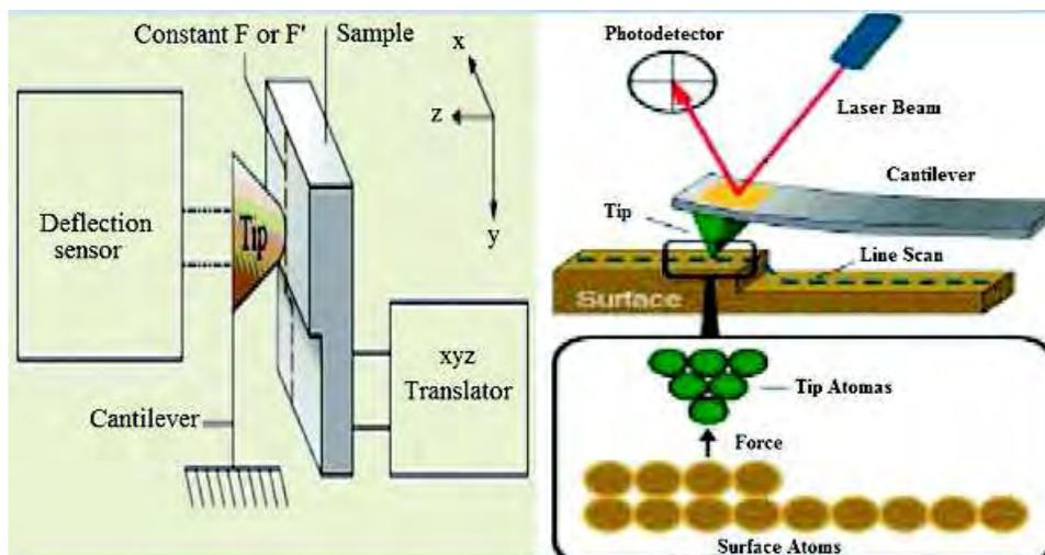
Fig. 4: Schematic Diagram of an AFM
