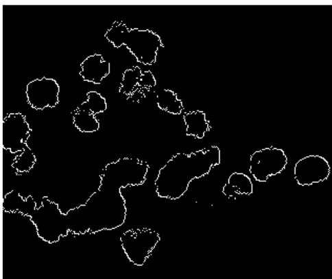
Fig. 10: Trace of Gold nanoparticles 20nm for its shape measurement in TEM image
