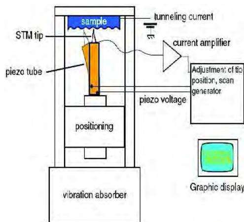
Fig. 2: Setup of a Scanning Tunneling Microscope
