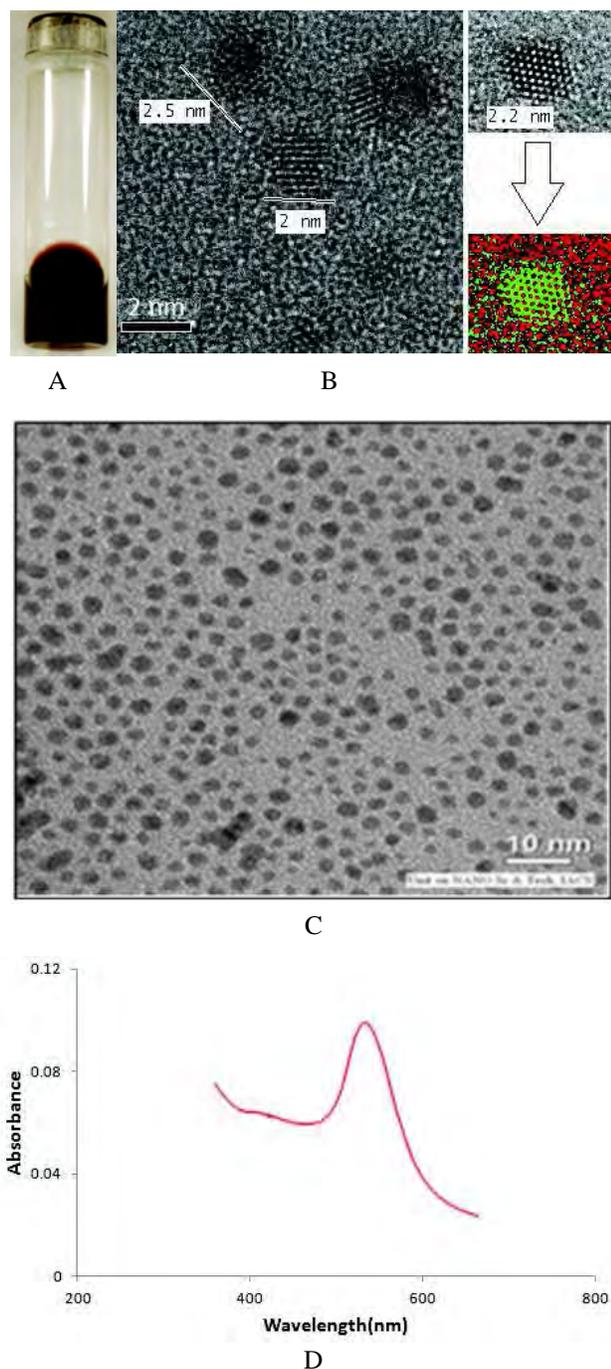
**Fig. 6:** A: Interface colour of thiol capped gold nanoparticle, B: TEM image of thiol capped GNP 2nm, C: TEM image of thiol capped GNP 3-5nm and D: Surface Plasmon peak of thiol capped gold nanoparticle
