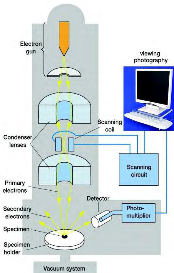
Fig. 3: Schematic Diagram of an SEM
