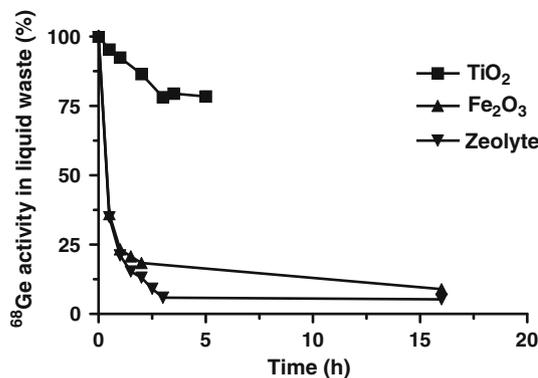
**Fig. 6** Recirculation system with <sup>68</sup>Ge waste in 1 M HCl. One gram of sorption material was enclosed, see Fig. 1. <sup>68</sup>Ge activity was quantified at indicated time points. Zeolite showed optimal sorption of <sup>68</sup>Ge activity within 4 h (>95%)
