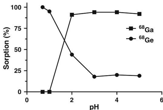
**Fig. 5** Sorption of <sup>68</sup>Ge activity on Zeolite was investigated as *f*(pH). After 24 h the samples were centrifuged. Supernatant was decanted and <sup>68</sup>Ge activity was quantified. Sorption of <sup>68</sup>Ge activity using Zeolite was optimal at pH <1
