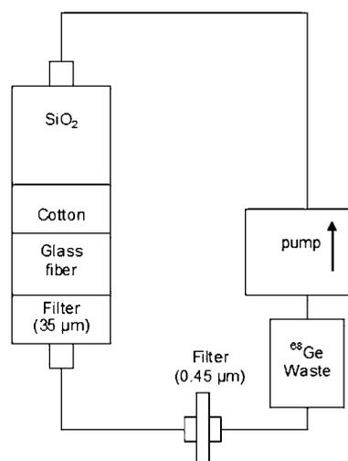
**Fig. 1** Recirculation system containing  $\pm 1$  g of  $\text{TiO}_2$ ,  $\text{Fe}_2\text{O}_3$  or Zeolite as sorption material enclosed with cotton, glass fiber and filters of 35 and  $0.45\ \mu\text{m}$ .  $^{68}\text{Ge}$  activity containing waste was recirculated at a flow rate of  $\pm 1$  mL/min. Samples of the circulating liquid were taken at indicated time points (see also Figs. 5, 6)
