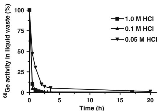
**Fig. 7** Since Zeolite showed an optimal sorption of  $^{68}\text{Ge}$  activity (Fig. 5), a column containing Zeolite ( $\pm 1$  g, Fig. 1) was tested with  $^{68}\text{Ge}$  waste in 0.05, 0.1 or 1.0 M HCl.  $^{68}\text{Ge}$  activity was quantified at indicated time points. Recirculation system using higher concentration of HCl showed high sorption of  $^{68}\text{Ge}$  activity at earlier time points
