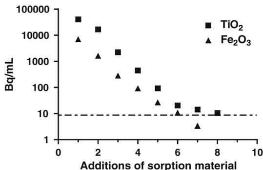
**Fig. 3** Samples of <sup>68</sup>Ge/<sup>68</sup>Ga generator eluate (50 mL) were used to investigate <sup>68</sup>Ge activity sorption on 0.5 g TiO<sub>2</sub> or 0.5 g Fe<sub>2</sub>O<sub>3</sub>. pH of the eluate was controlled by addition of phosphate buffer, final pH was ~8, and gently vortexed. Twenty-four hours after each addition, the 50 mL was centrifuged and a sample of the supernatant was collected to quantify <sup>68</sup>Ge activity
