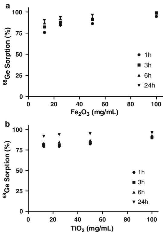
**Fig. 4** Complexation of <sup>68</sup>Ge activity of <sup>68</sup>Ge containing liquid waste (pH 8) with Fe<sub>2</sub>O<sub>3</sub> (a) or TiO<sub>2</sub> (b) as sorbent as function of time (1–24 h) and mass of sorbent (10–100 mg/mL)
