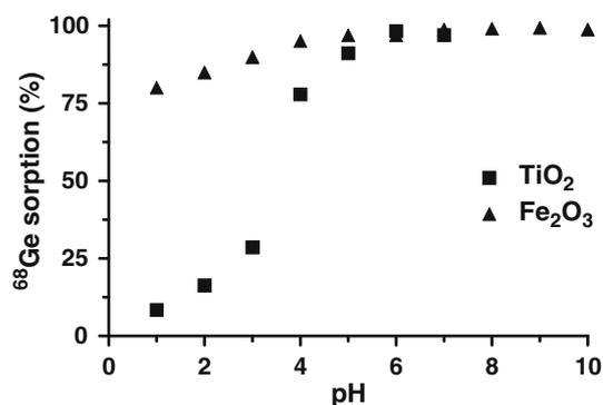
**Fig. 2** Sorption of  $^{68}\text{Ge}$  activity (10 kBq/g) on  $\text{Fe}_2\text{O}_3$  or  $\text{TiO}_2$  was investigated as  $f[\text{pH}]$ . After 24 h the samples were centrifuged. Supernatant was decanted and  $^{68}\text{Ge}$  activity was quantified. Sorption of  $^{68}\text{Ge}$  activity using  $\text{TiO}_2$  or  $\text{Fe}_2\text{O}_3$  was optimal at  $\text{pH} > 8$
