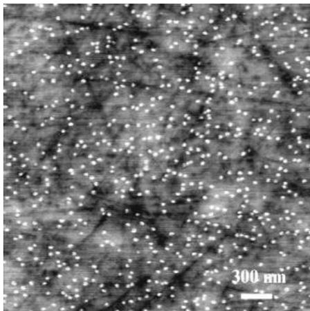
FIG. 7. The AFM analysis of the Ga nanodots on sapphire, showing a  $3 \times 3 \mu\text{m}^2$  AFM topograph.
