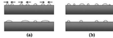
FIG. 10. Illustrations of possible Ga desorption models: (a) coalescence and (b) inhomogeneous desorption.
