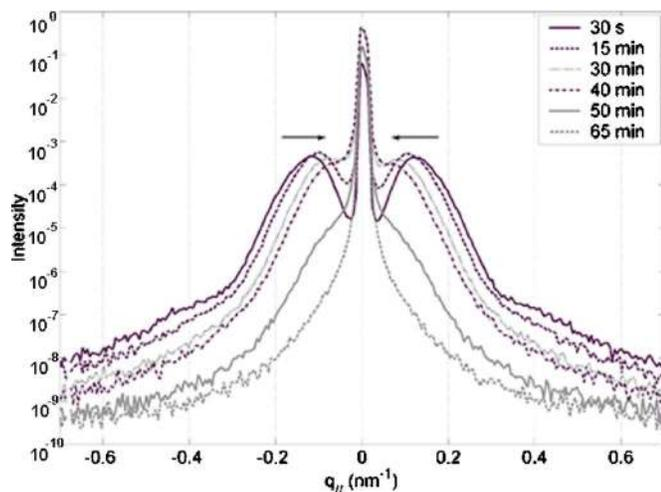
FIG. 4. Selected slices from the real-time GISAXS  $q_z$  scans at  $q_z = 0.5 \text{ nm}^{-1}$ , which shows the evolution of the surface morphology during desorption.
