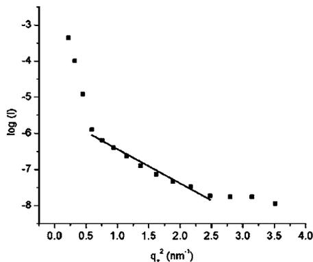
FIG. 5. The Guinier plot obtained from the GISAXS measurement taken 30 s after the Ga deposition has terminated. The solid line indicates the linear fit to the data.
