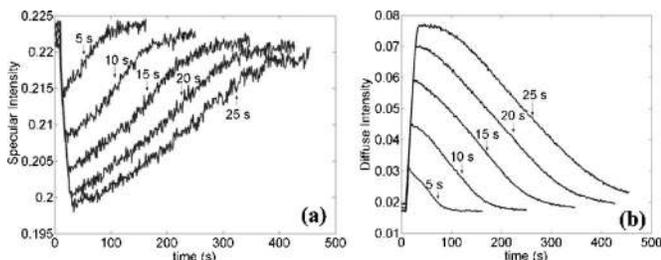
FIG. 8. The intensity evolution of the (a) near-specular and (b) diffuse parts of the GISAXS profiles in the predroplet regime as a function of Ga exposure time. The sapphire substrate temperature was  $700^\circ\text{C}$ .
