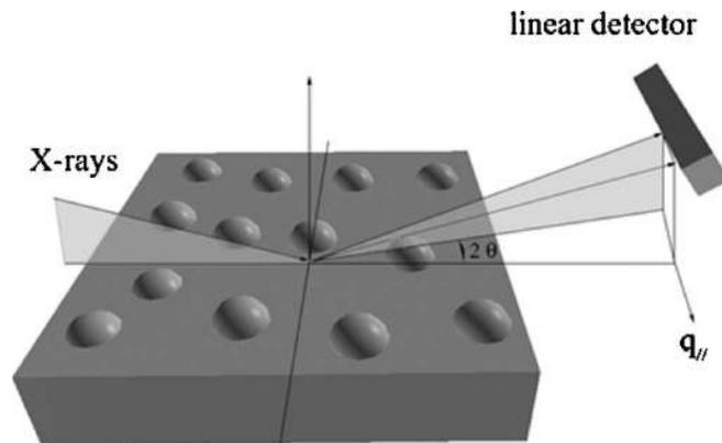
FIG. 1. The scattering geometry of the GISAXS. The linear detector is placed parallel to the sample surface to measure the scattering as a function of  $q_{||}$ .
