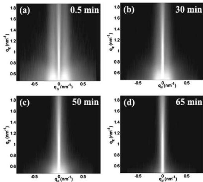
FIG. 3. Selected GISAXS  $q_z$  scans during desorption after 10 s Ga exposure.
