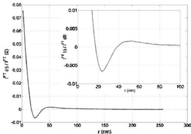
FIG. 6. Fourier transform of the measured GISAXS at  $q_z = 0.5 \text{ nm}^{-1}$ , which gives approximately the real-space electron density correlation. The peak at 50 nm indicates the average spacing between droplets and the intensity decay at smaller  $r$  values corresponds to the electron density distribution of individual droplets.
