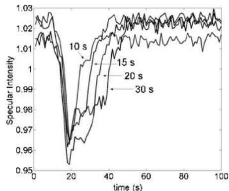
FIG. 9. The intensity evolution of the near-specular part of the GISAXS profile during Ga adsorption/desorption on GaN at  $700^\circ\text{C}$ .
