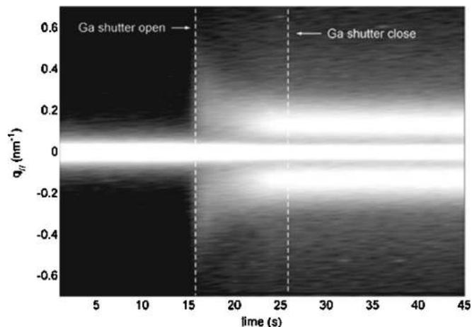
FIG. 2. The real-time GISAXS evolution of the sapphire surface during Ga adsorption and desorption at  $700^\circ\text{C}$ . The scan was taken at  $q_z = 1 \text{ nm}^{-1}$ .
