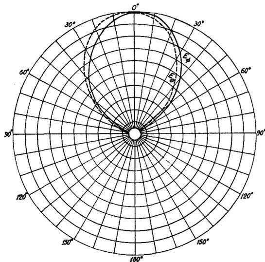
FIG. 3(b).  $E_\phi$  and  $E_\theta$  radiation patterns of the conical helix shown in Fig. 2a. Base is close to the "ground." Energy feed is at the base. Frequency, 150 Mc/sec.
