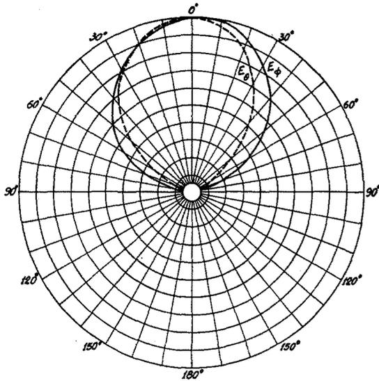
FIG. 4(b).  $E_\phi$  and  $E_\theta$  radiation patterns of the conical helix shown in Fig. 2b. Base is near the "ground." Feed is at the apex. Frequency, 200 Mc/sec.
