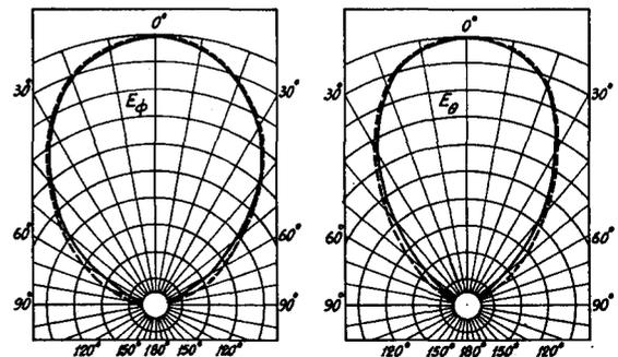
FIG. 10. Calculated (dotted lines) and observed (solid lines).  $E_{\phi}$  and  $E_{\theta}$  radiation patterns for the case shown in Fig. 3(c).
