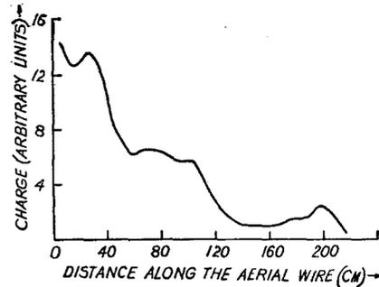
FIG. 7(c). Charge distribution along the length of the conical helix shown in Fig. 2. Base is close to the "ground" and feed is at the apex. Excitation frequency, 300 Mc/sec.
