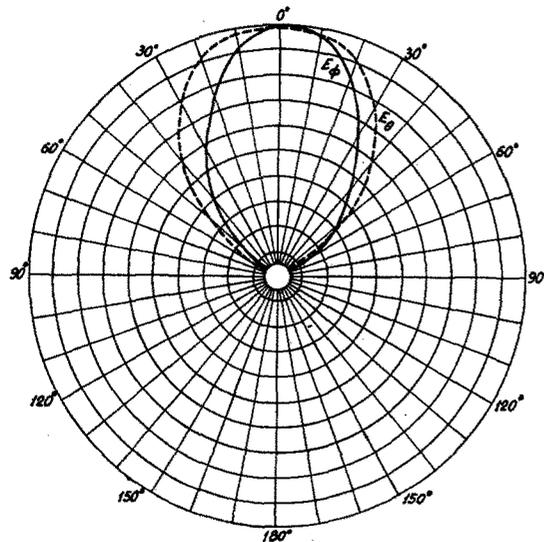
FIG. 4(c).  $E_\phi$  and  $E_\theta$  radiation patterns of the conical helix shown in Fig. 2b. Base is near the "ground." Feed is at the apex. Frequency, 300 Mc/sec.
