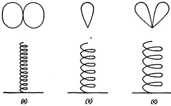
FIG. 1. Three types of radiation pattern of a cylindrical helix: (a) normal mode, (b) axial mode, (c) conical mode.
