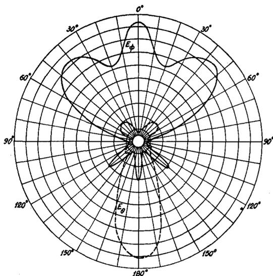
FIG. 5(b).  $E_\phi$  and  $E_\theta$  radiation patterns of the conical helix with the apex close to the "ground." Feed is at the base. Frequency, 200 Mc/sec.
