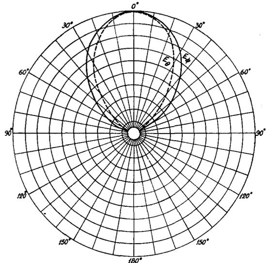
FIG. 3(c).  $E_\phi$  and  $E_\theta$  radiation patterns of the conical helix shown in Fig. 2a. Base is near the "ground." Feed is at the base. Frequency, 200 Mc/sec.
