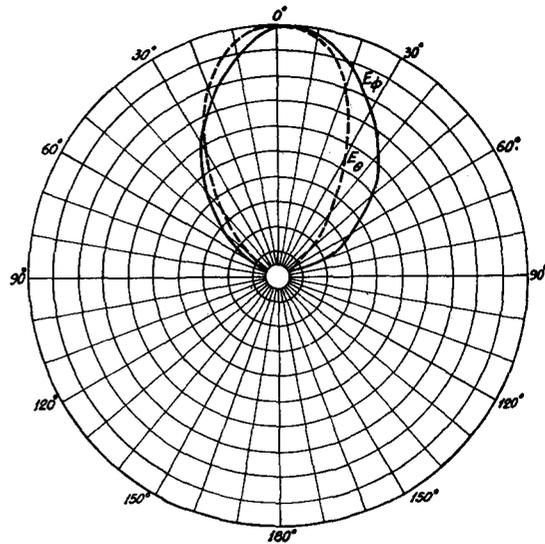
FIG. 4(a).  $E_\phi$  and  $E_\theta$  radiation patterns of the conical helix shown in Fig. 2b. Base is near the "ground." Feed is at the apex. Frequency, 150 Mc/sec.
