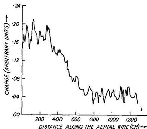
FIG. 8. Charge distribution along the length of the conical helix shown in Fig. 2. Base is close to the "ground" and feed is at the base. Excitation frequency, 200 Mc/sec.
