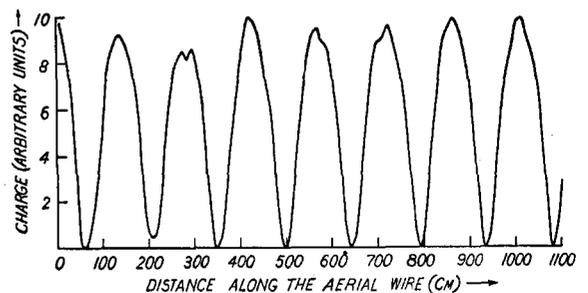
FIG. 7(a). Charge distribution along the length of the conical helix shown in Fig. 2. Base is close to the "ground" and feed is at the apex. Excitation frequency, 100 Mc/sec.
