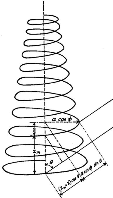
FIG. 9. Illustrating the calculation of the distance, from a point in the far zone, of an element  $ds$  of a loop of the helix with reference to the distance of the same point from the origin.
