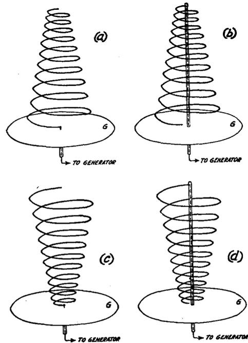
FIG. 2. Illustrating the different methods of feeding energy to the conical helix for different dispositions with respect to "ground." For case (a) the feed is at the base; (b) the feed is at the apex, the feeder passing axially through the helix; (c) feed at the apex; (d) feed is at the base, the feeder passing axially through the helix. Case (b) has the largest useful band width. For case (a) the band width is smaller, but the directivity is stronger.
