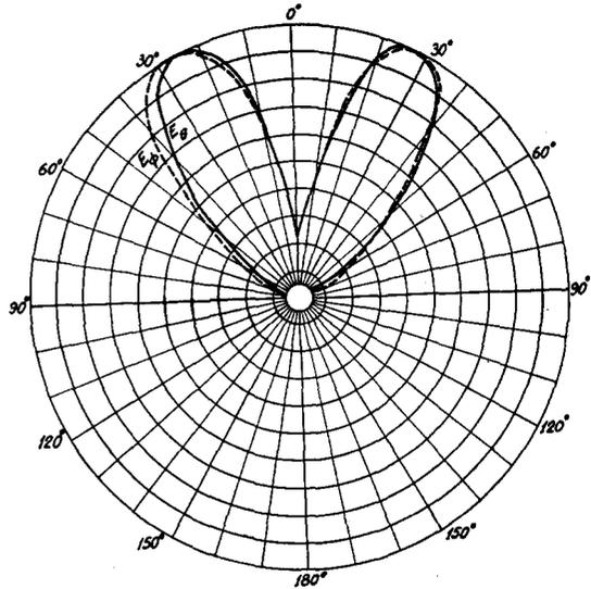
FIG. 3(e).  $E_\phi$  and  $E_\theta$  radiation patterns of the conical helix shown in Fig. 2a. Base is near the "ground." Feed is at the base. Frequency, 400 Mc/sec.
