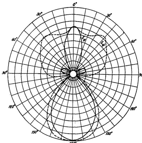
FIG. 6(a).  $E_\phi$  and  $E_\theta$  radiation patterns of the conical helix. Apex is close to the "ground" and feed is at the apex. Frequency, 150 Mc/sec.
