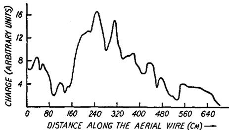
FIG. 7(b). Charge distribution along the length of the conical helix shown in Fig. 2. Base is close to the "ground" and feed is at the apex. Excitation frequency, 200 Mc/sec.
