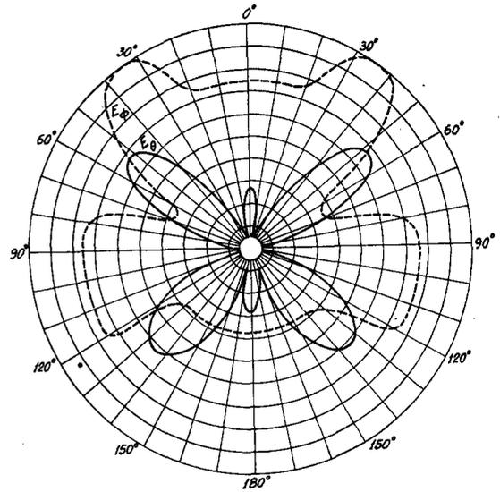
FIG. 6(c).  $E_\phi$  and  $E_\theta$  radiation patterns of the conical helix. Apex is close to the "ground" and feed is at the apex. Frequency, 300 Mc/sec.
