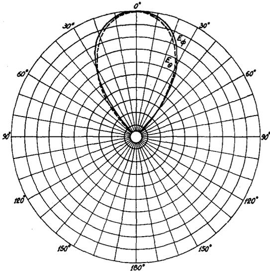
FIG. 3(d).  $E_\phi$  and  $E_\theta$  radiation patterns of the conical helix shown in Fig. 2a. Base is near the "ground." Feed is at the base. Frequency, 300 Mc/sec.
