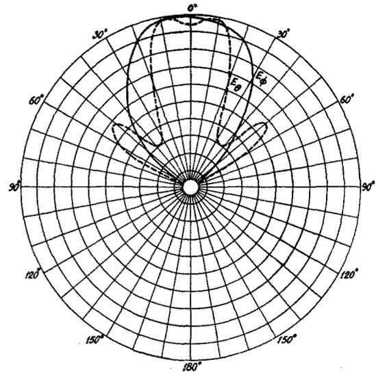
FIG. 4(d).  $E_\phi$  and  $E_\theta$  radiation patterns of the conical helix shown in Fig. 2b. Base is near the "ground." Feed is at the apex. Frequency, 450 Mc/sec.
