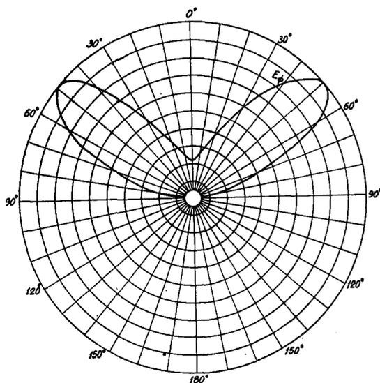
FIG. 5(c).  $E_\phi$  radiation pattern of the conical helix with the apex close to the "ground." Feed is at the base. Frequency, 300 Mc/sec.
