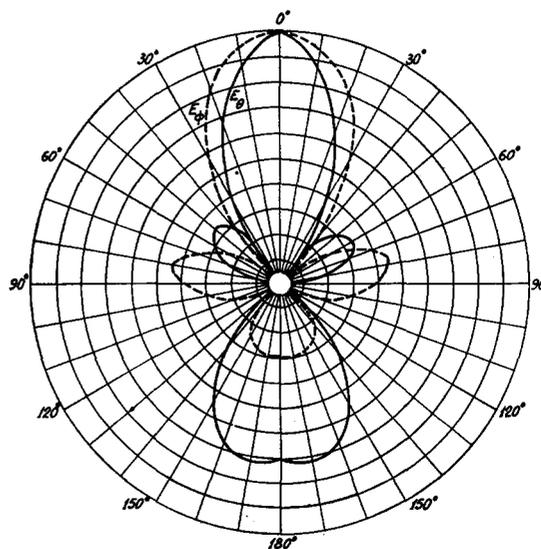
FIG. 6(b).  $E_\phi$  and  $E_\theta$  radiation patterns of the conical helix. Apex is close to the "ground" and feed is at the apex. Frequency, 200 Mc/sec.
