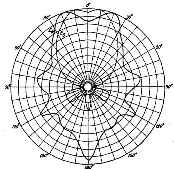
FIG. 5(a).  $E_\phi$  and  $E_\theta$  radiation patterns of the conical helix with the apex close to the "ground." Feed is at the base. Frequency, 150 Mc/sec.
