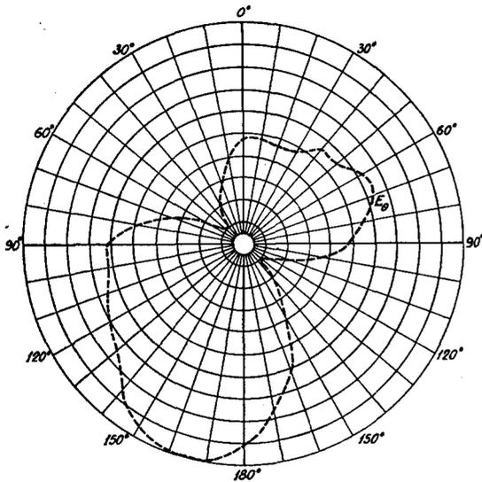
FIG. 3(a).  $E_\theta$  radiation pattern of the conical helix shown in Fig. 2a. Base is close to the "ground." Energy feed is at the base. Frequency, 120 Mc/sec.
