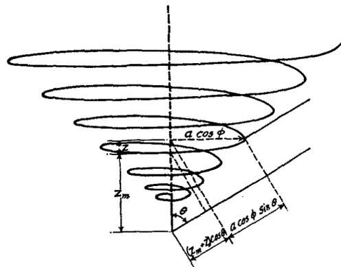
FIG. 5. Illustrating the calculation of the distance from a point in the far zone, of an element  $ds$  of a loop of the helix with reference to the distance of the same point from the origin.
