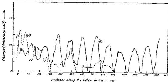
FIG. 3. Charge distribution along the length of the conical helix shown in Fig. 1. The zero point of the abscissa is at *B*. Excitation frequency, (a) 100 Mc/sec, (b) 220 Mc/sec.
