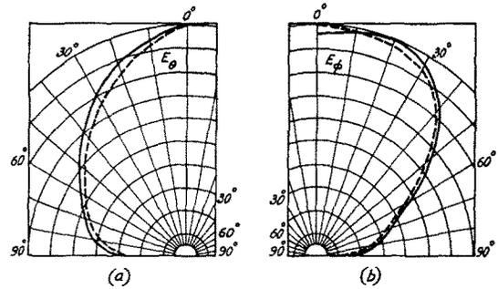
Fig. 6. Calculated (dotted lines) and experimentally observed (solid lines) radiation patterns of (a)  $E_\theta$  and (b)  $E_\phi$ . Frequency, 300 Mc/sec.
