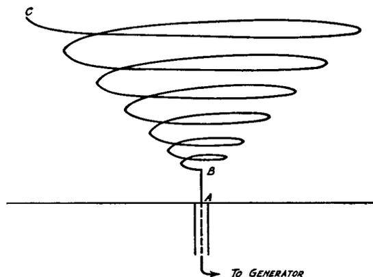
FIG. 1. Illustrating the method of feeding energy to the conical helix with respect to "ground."
