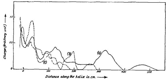
FIG. 4. Charge distribution along the length of the conical helix shown in Fig. 1. The zero point of the abscissa is at *B*. Excitation frequency, (a) 300 Mc/sec, (b) 400 Mc/sec, (c) 500 Mc/sec.
