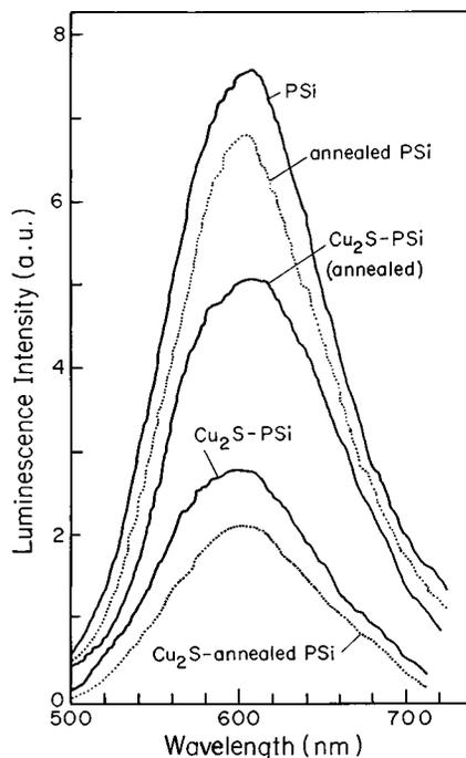
FIG. 5. Luminescence from PSi through a top film of  $\text{Cu}_2\text{S}$ , compared with that from a bare PSi surface. Data for materials prepared under different conditions, as indicated in the figure, are presented.
