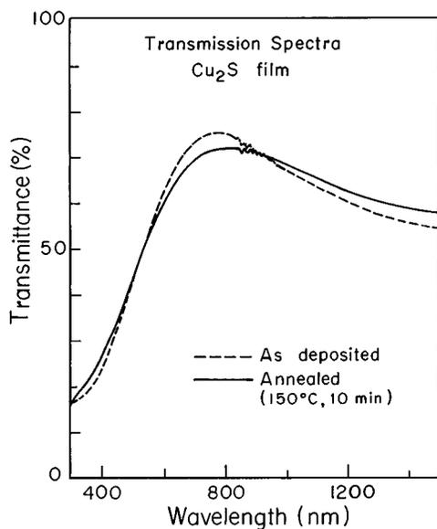
FIG. 2. Optical transmission spectra for the as-deposited and the 150 °C annealed  $\text{Cu}_2\text{S}$  films.
