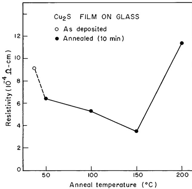
FIG. 1. Resistivity of the as-deposited and the annealed  $\text{Cu}_2\text{S}$  films on glass.
