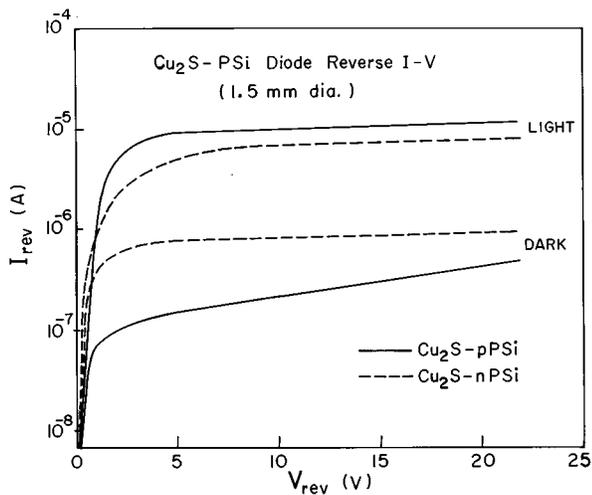
FIG. 4. Reverse  $I$ - $V$  data for  $\text{Cu}_2\text{S}$ -PSi diodes in the dark and in the presence of light. Si substrate resistivity for  $p$ - and  $n$ -type PSi are 40 and 50  $\Omega$  cm, respectively.
