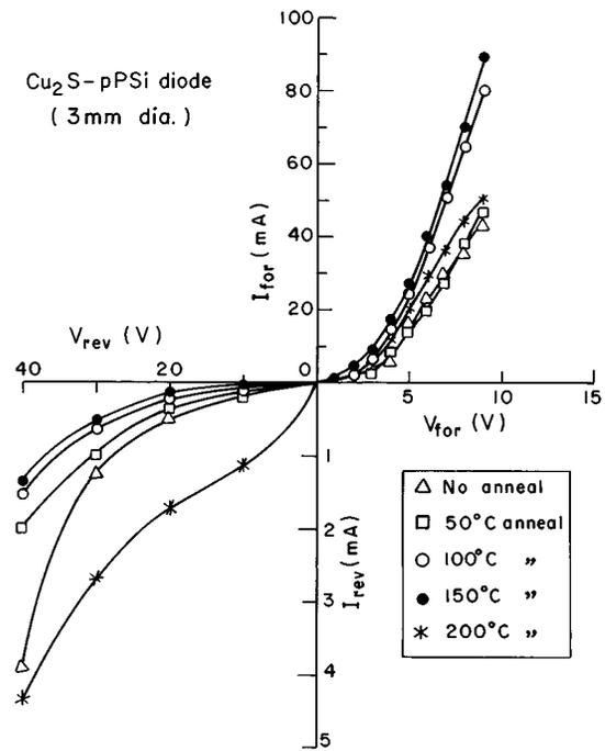
FIG. 3.  $I$ – $V$  characteristics of  $\text{Cu}_2\text{S}$ – $p$ -type P*Si* diodes. The data for devices using as-deposited  $\text{Cu}_2\text{S}$  film as well as films annealed at different temperatures are being shown.
