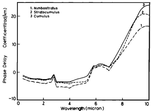
Figure 5. Phase delay coefficients for different fog models.
