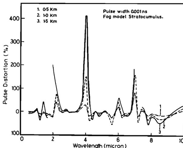
**Figure 2.** Distortion of a pulse with width 0.001 ns for the stratocumulus fog model over different path lengths.
