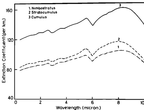
Figure 4. Extinction coefficients for different fog models.
