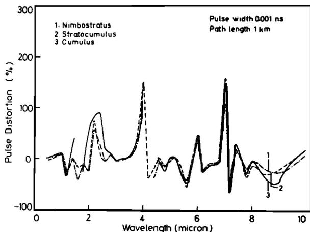
**Figure 1.** Pulse distortion over a 1-km path length for pulse width of 0.001 ns for different fog models.
