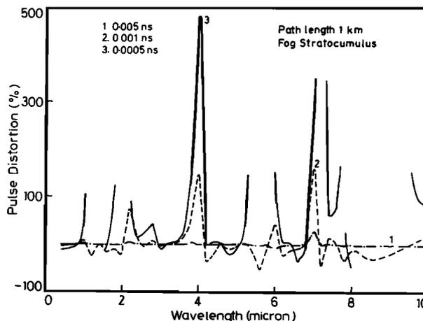
**Figure 3.** Pulse distortion over a 1-km path length for the stratocumulus fog model for different pulse widths.
