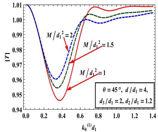
Fig. 12.  $|T|$  against  $k_0^{(1)}d_1$  for different values of surface tension.
