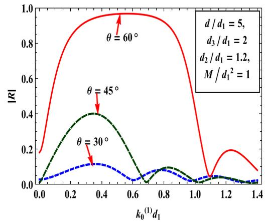
Fig. 7.  $|R|$  for different values of angles in presence of surface tension.
