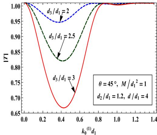
Fig. 14.  $|T|$  for different values of depth of the asymmetric trench in presence of surface tension.
