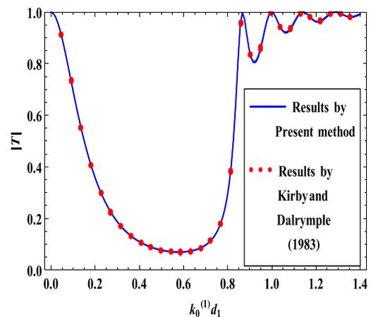
Fig. 3.  $|T|$  against  $k_0^{(1)}d_1$  for  $d_3/d_1 = 3.0$ ,  $d_2/d_1 = 1.0$ ,  $d/d_1 = 10.0$ ,  $M/d_1^2 = 0$ ,  $\theta = 45^\circ$ .
