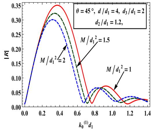
Fig. 11.  $|R|$  against  $k_0^{(1)}d_1$  for different values of surface tension.
