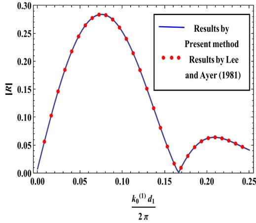
Fig. 4.  $|R|$  against  $\frac{k_0^{(1)} d_1}{2\pi}$  for  $\frac{d_3}{d_1} = 2.0$ ,  $\frac{d_2}{d_1} = 1.0$ ,  $\frac{d}{d_1} = 2.5$ ,  $\frac{M}{d_1^2} = 0$ ,  $\theta = 0^\circ$ .
