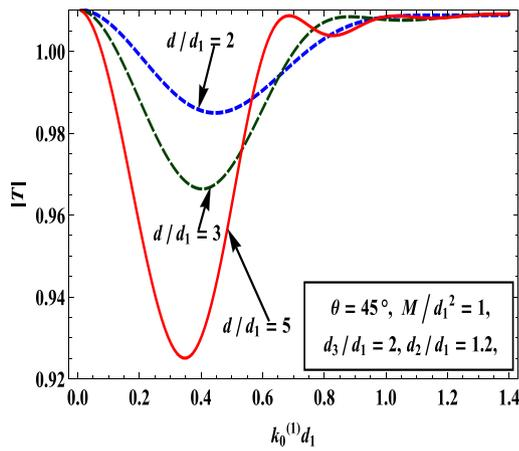
Fig. 10.  $|T|$  for different values of width of the asymmetric trench in presence of surface tension.
