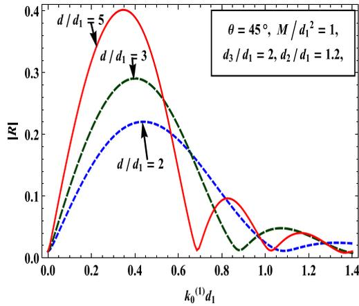
Fig. 9.  $|R|$  for different values of width of the asymmetric trench in presence of surface tension.
