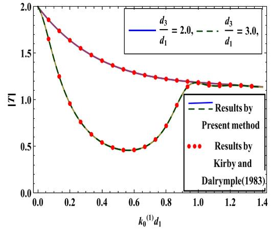
Fig. 6.  $|T|$  against  $k_0^{(1)} d_1$  for  $\frac{d_2}{d_1} = 2.0$ ,  $\frac{d}{d_1} = 5.0$ ,  $\frac{M}{d_1^2} = 0$ ,  $\theta = 45^\circ$ .
