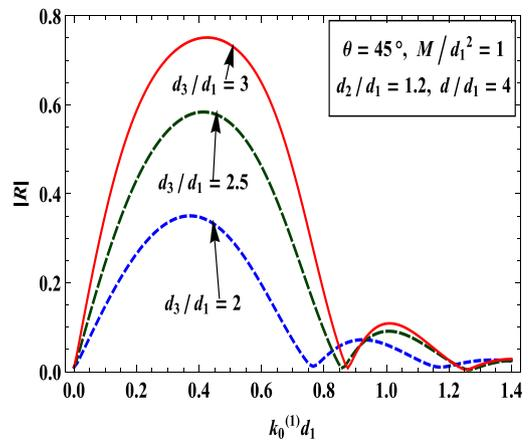
Fig. 13.  $|R|$  for different values of depth of the asymmetric trench in presence of surface tension.
