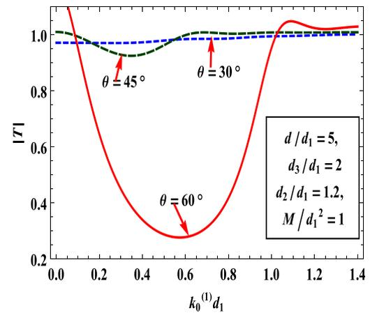
Fig. 8.  $|T|$  for different values of angles in presence of surface tension.
