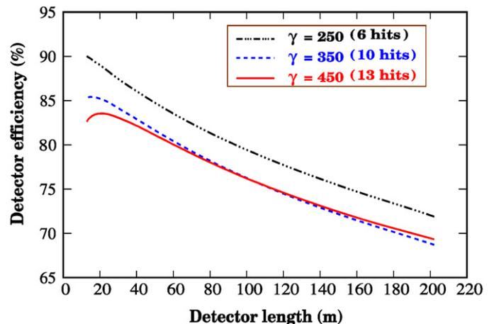
Fig. 2. Detector efficiency for  $\gamma = 250, 350, 450$ . The corresponding cuts on muon hits used are 6, 10 and 13, respectively.
