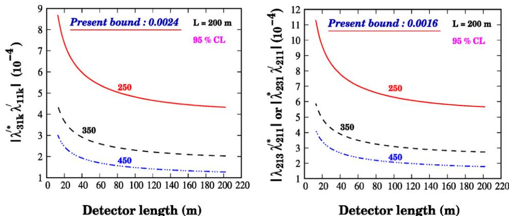
Fig. 8. Bounds on  $|\lambda'_{31k} \lambda'_{11k}|$ ,  $k = 2, 3$  ( $|\lambda_{231} \lambda_{211}|$  or  $|\lambda_{213} \lambda_{211}|$ ) versus detector size at 95% CL for zero observed events is depicted in left (right) panel for  $\gamma = 250, 350, 450$ . The bounds scale as  $(\bar{m}/100 \text{ GeV})^2$ . The results are for a five-year run for a 5 kT Fe detector placed at a distance of 200 m from the front end of the storage ring for  $^8\text{B}$  beta-beam flux.
