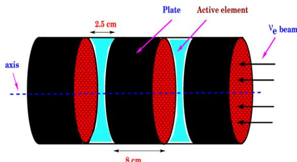
Fig. 1. A schematic diagram of the proposed detector (a part only). The incoming  $\nu_e$  beam may have a very small contamination of neutrinos of other flavours in the presence of lepton flavour violating interactions.
