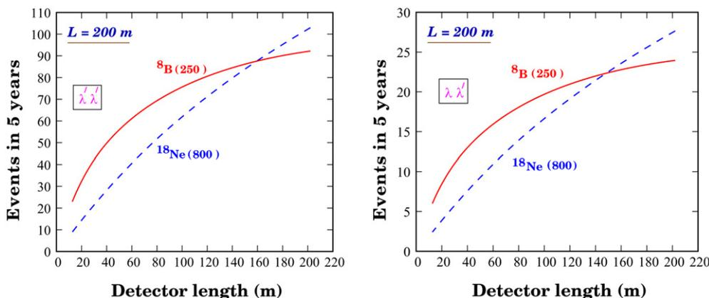
Fig. 9. Comparison of the muon signal event rates as a function of the detector length for a 5 kT iron calorimeter placed at a distance of 200 m from the storage ring for  $\gamma = 800$  (250) with  $^{18}\text{Ne}$  ( $^8\text{B}$ ). The left and right panels correspond to  $\lambda'\lambda'$  and  $\lambda\lambda'$  driven processes, respectively.
