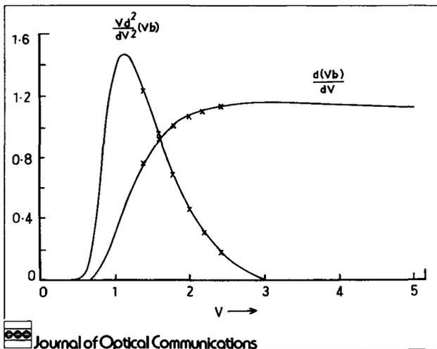
Fig. 1:  $d(Vb)/dV$  and  $V d^2(Vb)/dV^2$  versus  $V$  for the fundamental mode of weakly-guiding step index fiber (x our theoretical results based on Chebyshev technique; — theoretical results [13])
