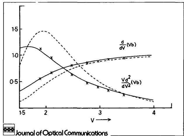
Fig. 2:  $d(Vb)/dV$  and  $V d^2(Vb)/dV^2$  versus  $V$  for the fundamental mode of weakly-guiding parabolic index fiber (x our theoretical results based on Chebyshev technique; — theoretical results [1]; - - - theoretical results based on Gaussian approximation [1])
