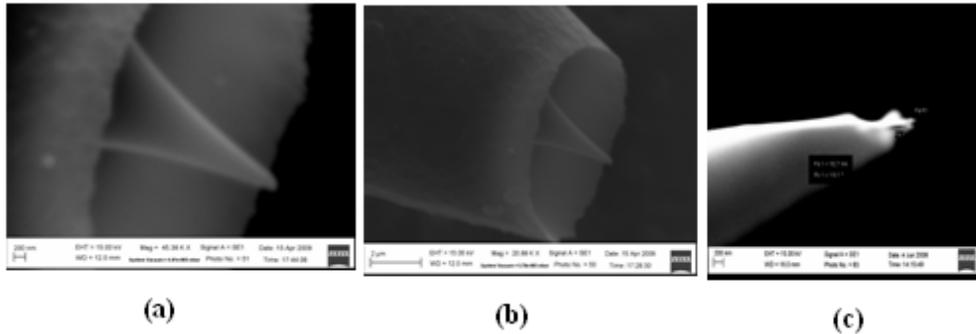
Fig. 2. (a) and (b) are SEM images of NNP with different resolutions, (c) is SEM image of NNP made by single step meniscus rise based chemical etching under similar conditions. The rim at the base of the nanoprobe likely to be part of the capillary ring left after completion of etching. The scale bars are (a) 200 nm, (b) 2 μm, and (c) 200 nm.
