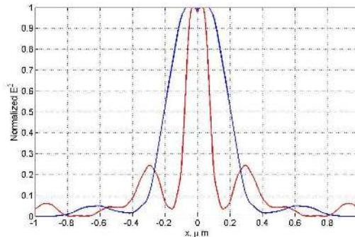
Fig. 4. Normalized near field distribution for NNP (—) and CNP (—) at 100 nm from probes tip.
