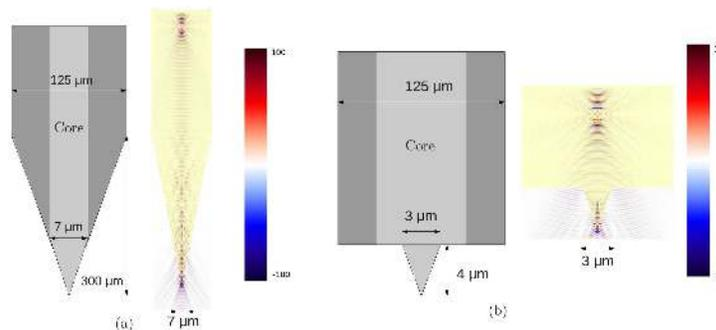
Fig. 3. plots FDTD simulation results for optical field propagation and distribution in fiber with nanoprobe illuminated by similar source but different amplitudes. The adjacent color bars are to estimate magnitude of the field in the probes. The schematic of single-mode fibers (core  $7\mu\text{m}$ , diameter  $125\mu\text{m}$ ) with probe present respective design.
