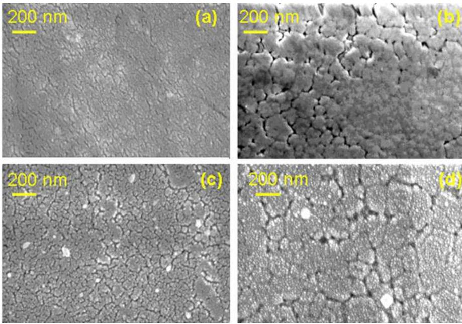
FIG. 2. Surface morphologies of (a) PLT15, (b) 96.4 PLT15-3.6 CFO, (c) 94.06 PLT15 - 5.94 CFO, and (d) 88.26 PLT15 - 11.74CFO composite thin films on transparent sapphire (0001) substrates.
