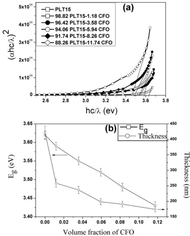
FIG. 6. (a)  $(\alpha h\nu)^2$  vs  $(h\nu)$  plots for all these films, (b) the variation of optical band gap ( $E_g$ ) with CFO volume contents and film thickness in  $(1-x)$  PLT15- $x$  CFO composite thin films.
