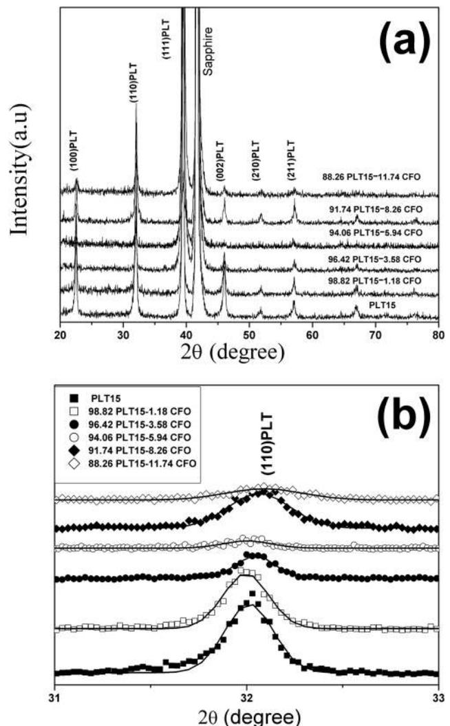
FIG. 1. (a) XRD patterns of PLT15 and  $(1-x)$  PLT15- $x$  CFO composite films on sapphire substrate. (b) Slow scanned (110) x-ray diffraction peaks.
