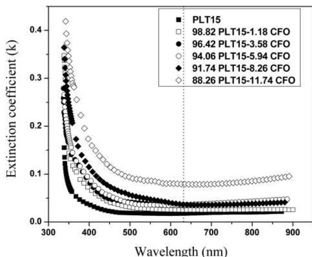
FIG. 5. Plot of  $k$  as a function of  $\lambda$  for PLT15, and  $(1-x)$  PLT15- $x$  CFO composite thin films.
