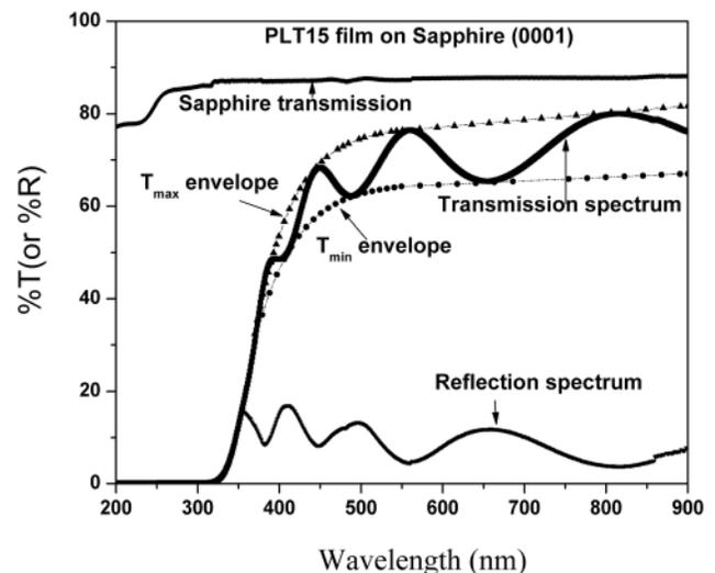
FIG. 3. Transmittance and reflectance spectra and the  $T_{\max}$  and  $T_{\min}$  envelopes for undoped PLT film on a completely transparent sapphire (0001) substrate.
