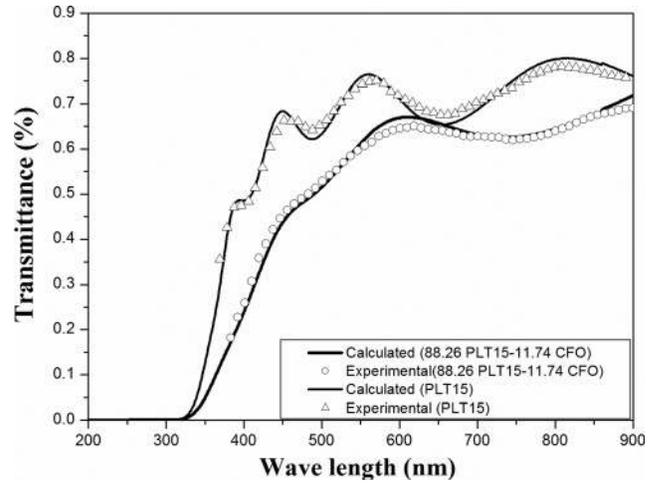
FIG. 7. Computed transmittance data with experimental values for 88.26 PLT15-11.74 CFO composites thin film.
