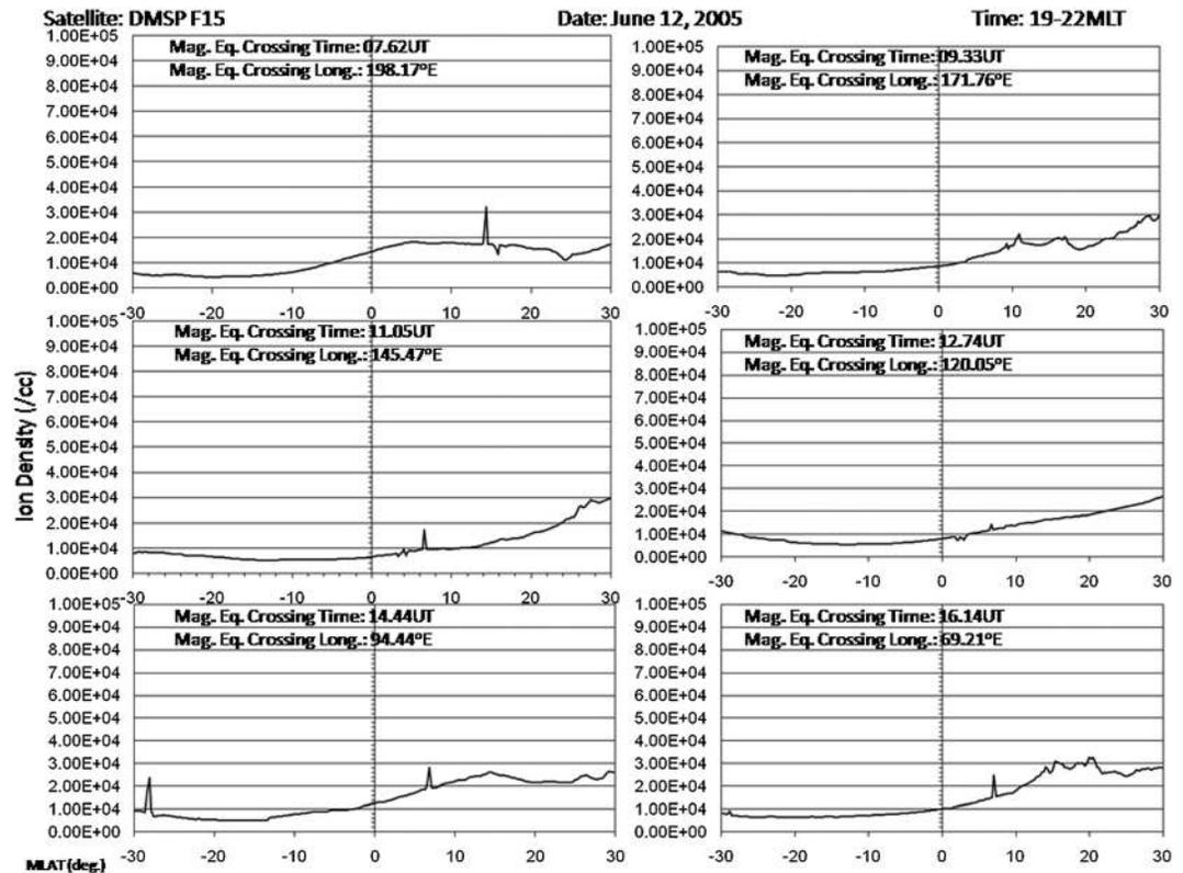
Figure 2. Plots of total ion density (/cc) observed by DMSP F15 during 12 June 2005.
