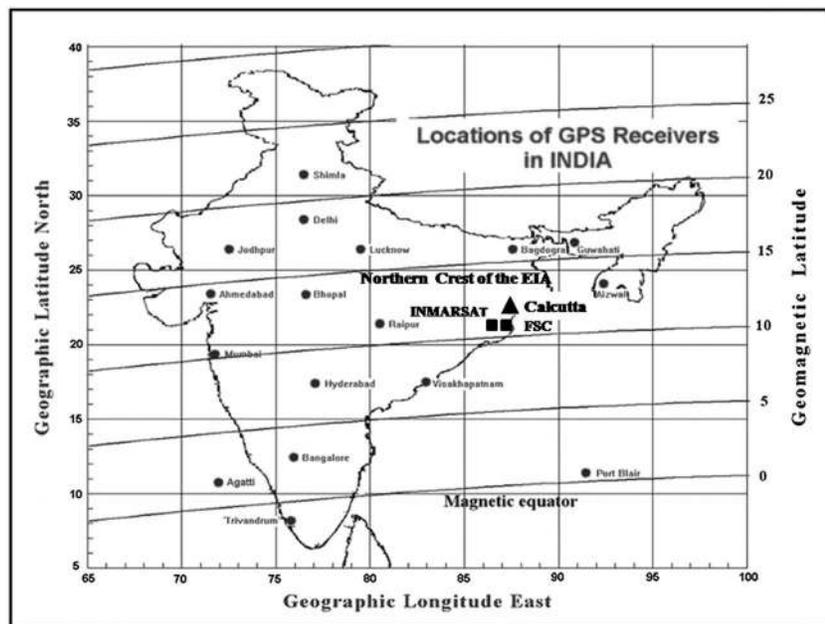
Figure 8. Map of India showing the location of GAGAN reference stations, subionospheric points of Inmarsat, and FSC. The magnetic equator and the northern crest of the equatorial anomaly are also indicated.
