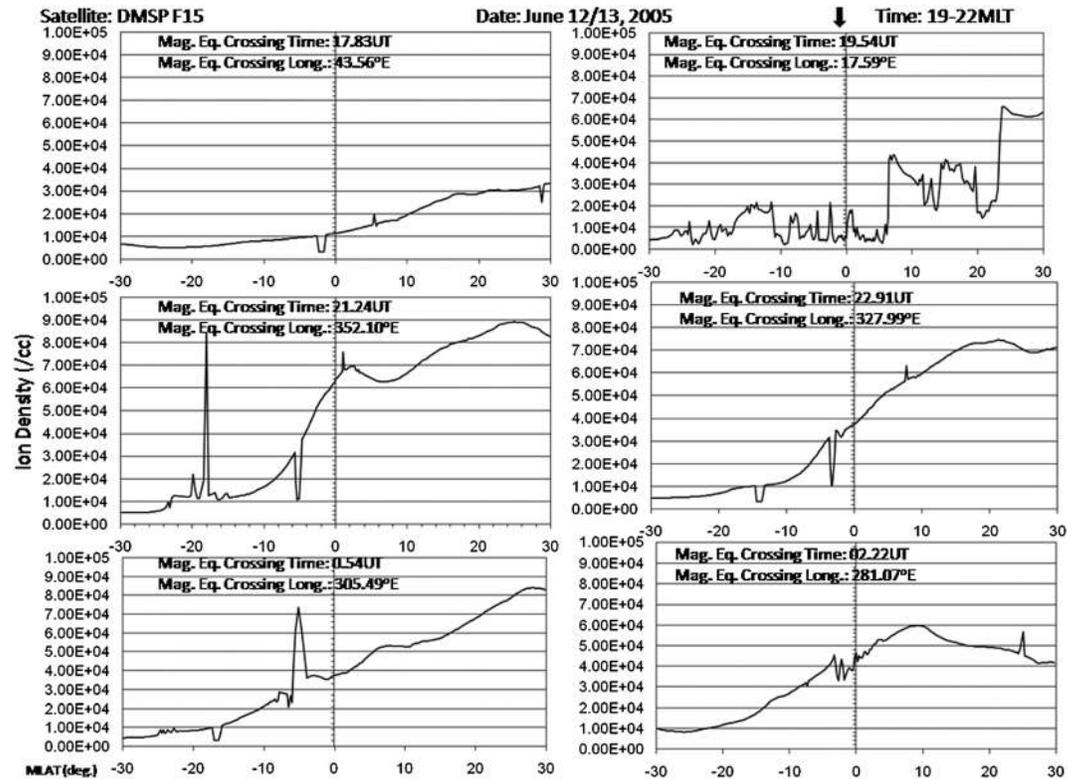
**Figure 3.** Plots of total ion density (/cc) observed by DMSP F15 during 12–13 June 2005. The black arrow indicates the frame showing the presence of irregularities.
