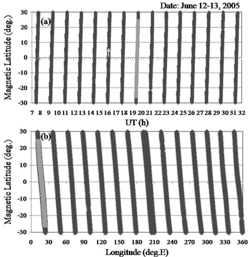
**Figure 4.** Presence of irregularities (indicated by the light grey portion) in DMSP tracks represented in (a) time and (b) longitude during the intense magnetic storm of 12–13 June 2005. The white arrow in Figure 4a indicates the time of southward IMF  $B_z$  crossing  $-10$  nT. ESF generation is at 19:54 UT, 3.53 h after the time of IMF  $B_z$  crossing  $-10$  nT at 16:01 UT, at a longitude  $17.64^\circ$  whose local time is 20:72.
