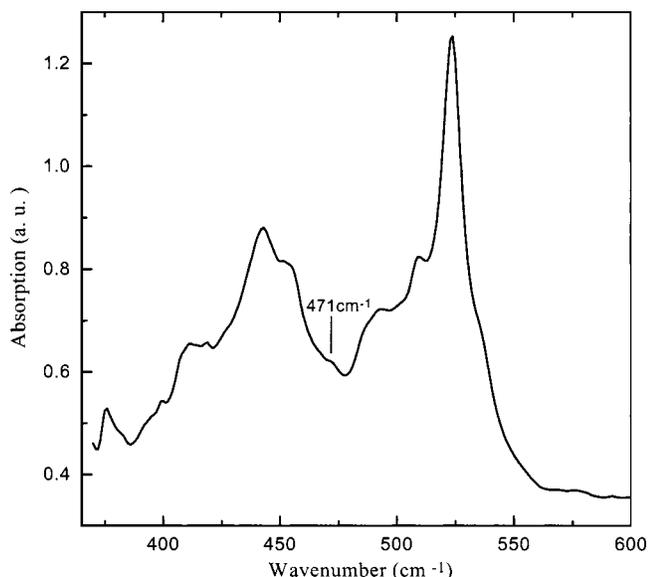
FIG. 1. FTIR absorption spectrum for LPE GaAsN.
