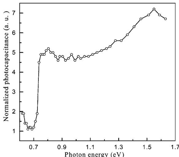
FIG. 4. 10 K phot capacitance spectrum for LPE GaAsN.
