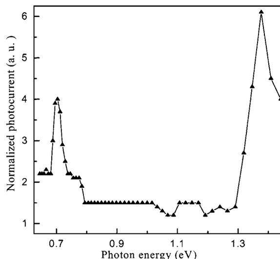
FIG. 3. Room-temperature photocurrent spectrum for LPE GaAsN.
