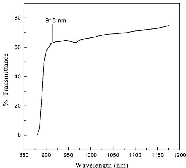
FIG. 2. Room-temperature optical transmission spectrum for LPE GaAsN.
