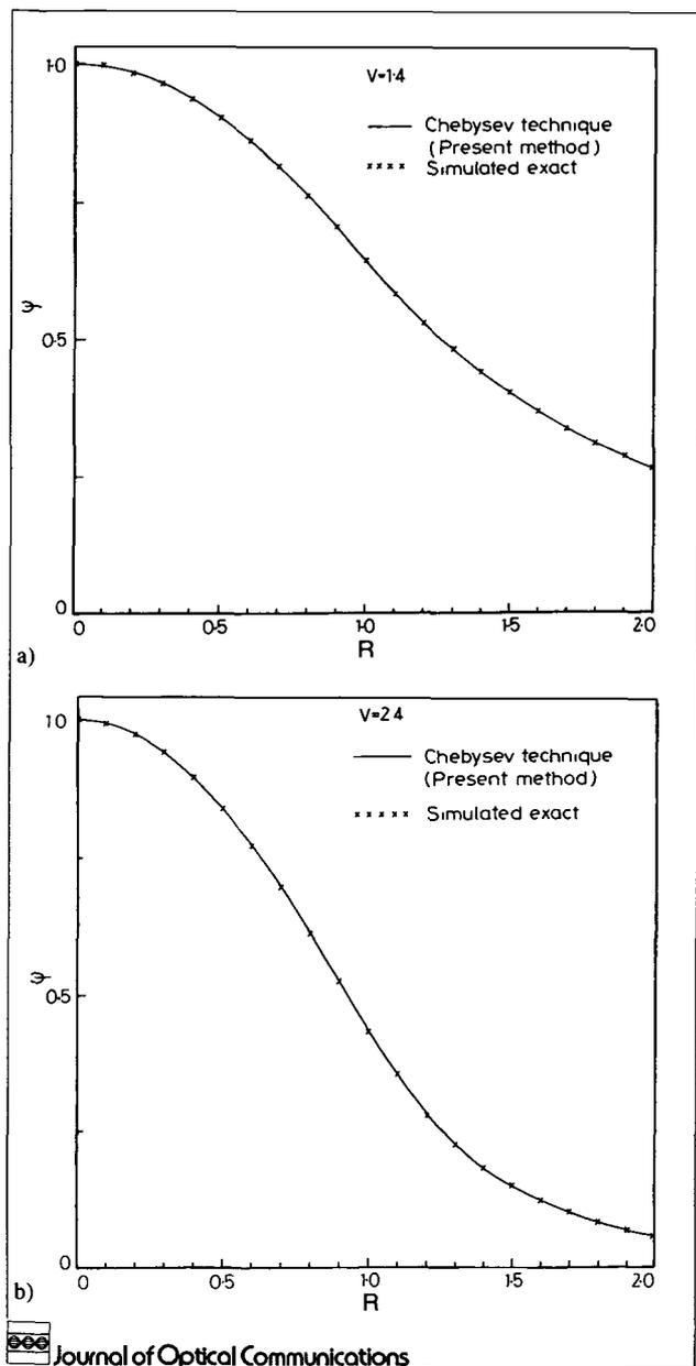
Figure 1 : The fundamental modal field  $\psi$  as a function of normalised radius  $R$  for a step index fiber with (a)  $V = 1.4$  and (b)  $V = 2.4$
