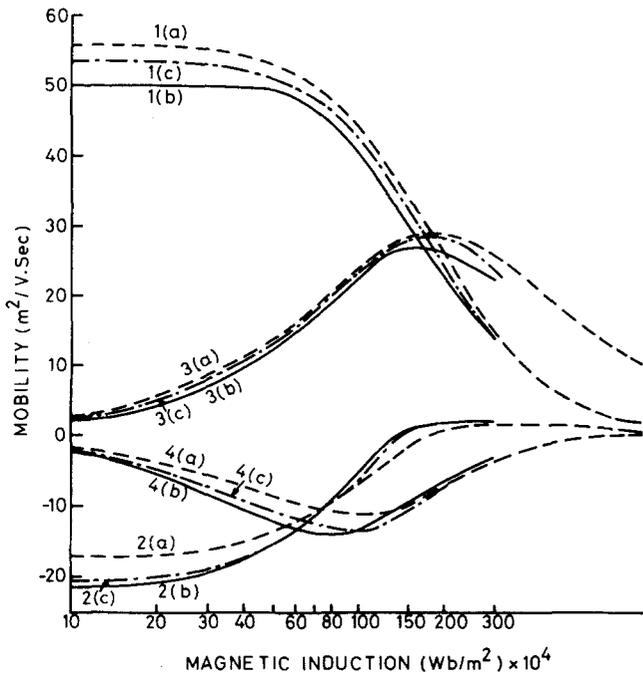
FIG. 1. Complex mobility of  $n$ -InSb at 77°K at different magnetic fields for a frequency of 10 GHz. Curves numbered 1–4 represent, respectively, the components of the mobility tensor:  $\mu_{xx}$ ,  $\mu_{xi}$ ,  $\mu_{yy}$ , and  $\mu_{yi}$ . Letters in parenthesis indicate, respectively, the values obtained from the Drude theory, (a); and present calculations with  $E_1 = 7.2$  eV, (b); and  $E_1 = 30$  eV, (c).
