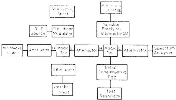
FIG. 1. Setup for the measurement of resonator  $Q$ .
