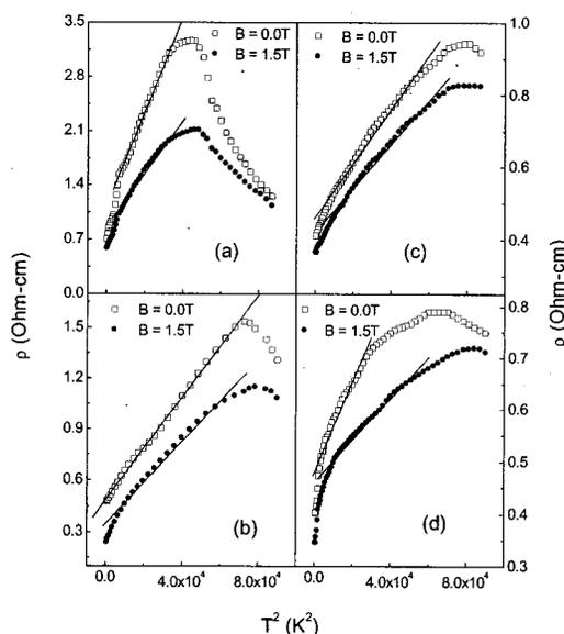
FIG. 4. Linear fit of the low temperature (low temperature  $T < T_p$ , FM region) resistivity data with the  $T^2$  term [Eq. (1)] in the absence ( $B=0$ ) and presence ( $B=1.5$  T) of the magnetic field ( $B$ ) for the samples  $\text{La}_{0.7}\text{Ca}_{0.3-y}\text{Na}_y\text{MnO}_3$  with (a)  $y=0.0$ , (b)  $y=0.05$ , (c)  $y=0.1$ , (d)  $y=0.15$ .
