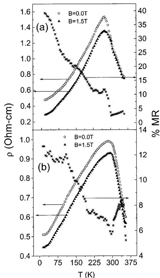
FIG. 3. Variation of resistivity in the absence ( $B=0.0$  T) and presence ( $B=1.5$  T) of the magnetic field ( $B$ ) and %MR (for  $B=1.5$  T) with temperature for the sample  $\text{La}_{0.7}\text{Ca}_{0.3-y}\text{Na}_y\text{MnO}_3$  with  $y =$  (a) 0.05 and (b) 0.15.
