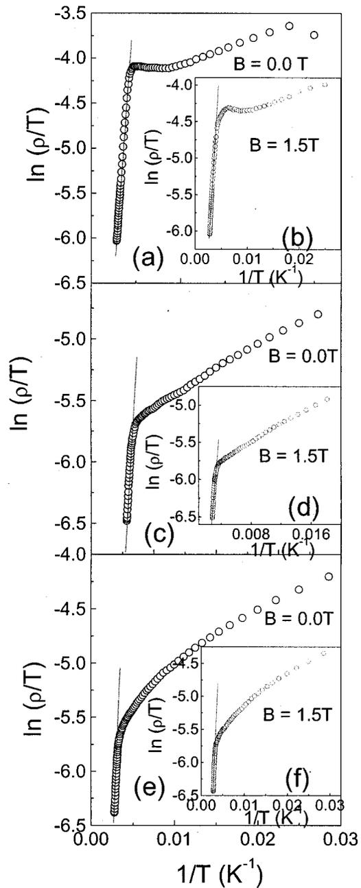
FIG. 6. Variation of  $\ln(\rho/T)$  as a function of inverse temperature  $1/T$  for the sample  $\text{La}_{0.7}\text{Ca}_{0.3-y}\text{Na}_y\text{MnO}_3$  with  $y = 0.0$  for (a) and (b);  $y = 0.10$  for (c) and (d);  $y = 0.15$  for (e) and (f). Inset graphs (b), (d), and (f) shows the plot with field  $B = 1.5$  T. Solid lines are the best fit to the SPH model [Eq. (2)].
