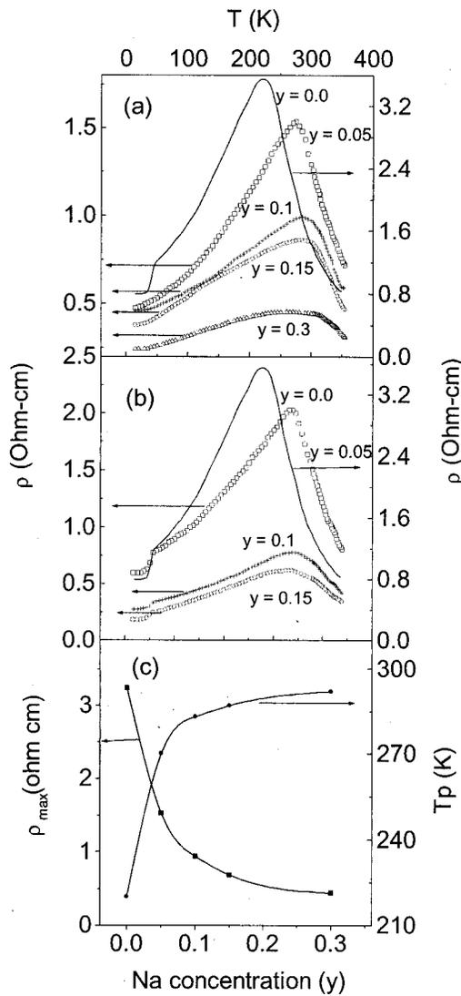
FIG. 1. Thermal variation of resistivity ( $\rho$ ) of (a)  $\text{La}_{0.7}\text{Ca}_{0.3-y}\text{Na}_y\text{MnO}_3$  ( $0.0 \leq y \leq 0.3$ ) and (b)  $\text{La}_{0.7}\text{Ca}_{0.3-y}\text{K}_y\text{MnO}_3$  ( $0.0 \leq y \leq 0.15$ ) at zero applied field. (c) Maximum resistivity ( $\rho_{\max}$ ) and metal insulator transition (MIT) temperature  $T_p$  as a function of doping concentration ( $y$ ) showing clearly the saturation of  $\rho_{\max}$  and  $T_p$  after a certain doping level.
