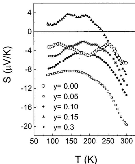
FIG. 8. Thermal variation of the Seebeck coefficient ( $S$ ) of  $\text{La}_{0.7}\text{Ca}_{0.3-y}\text{Na}_y\text{MnO}_3$  with  $y=0, 0.05, 0.1, 0.15,$  and  $0.3$  without applying the magnetic field.
