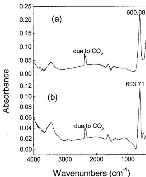
FIG. 5. Infrared spectra of two typical samples  $\text{La}_{0.7}\text{Ca}_{0.3-y}\text{Na}_y\text{MnO}_3$  with (a)  $y = 0.0$  and (b)  $y = 0.1$  in the KBr pellet at room temperatures from where optical phonon frequency was estimated and compared with that obtained from the conductivity data (from Debye temperature).
