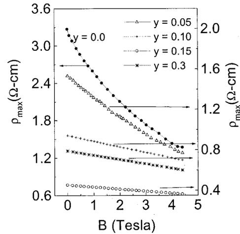
FIG. 2. Variation of maximum resistivity ( $\rho_{\max}$ ) at the metal insulator transition temperature ( $T_p$ ) of the  $\text{La}_{0.7}\text{Ca}_{0.3-y}\text{Na}_y\text{MnO}_3$  ( $0.0 \leq y \leq 0.3$ ) samples with an increase of magnetic field ( $B = 0 - 4.4$  T).
