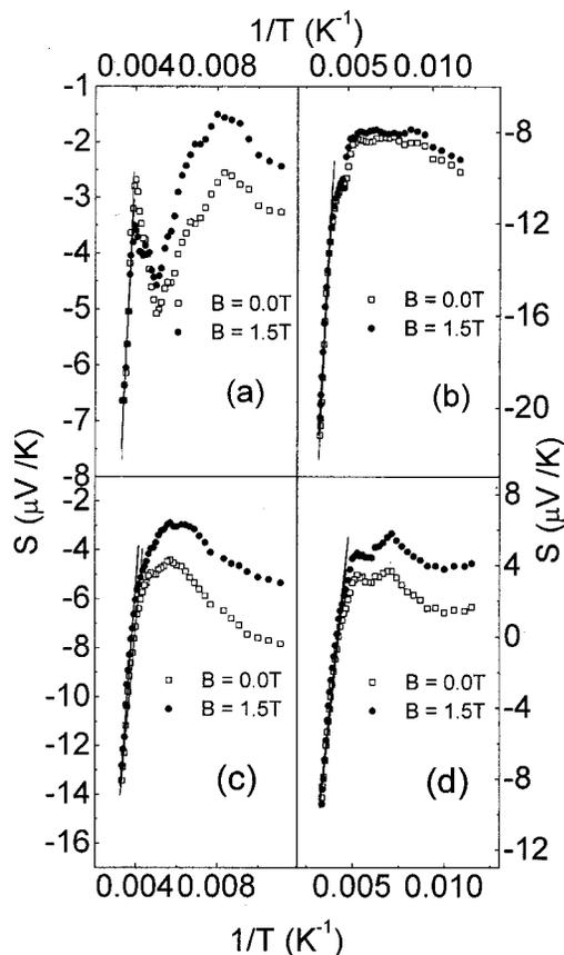
FIG. 10. The Seebeck coefficient  $S$  vs  $1/T$  plot for four different  $\text{La}_{0.7}\text{Ca}_{0.3-y}\text{Na}_y\text{MnO}_3$  samples with (a)  $y=0.0$ , (b)  $0.05$ , (c)  $0.1$ , and (d)  $0.15$ . Solid lines are the best-fit lines to the Mott's model [Eq. (4)].
