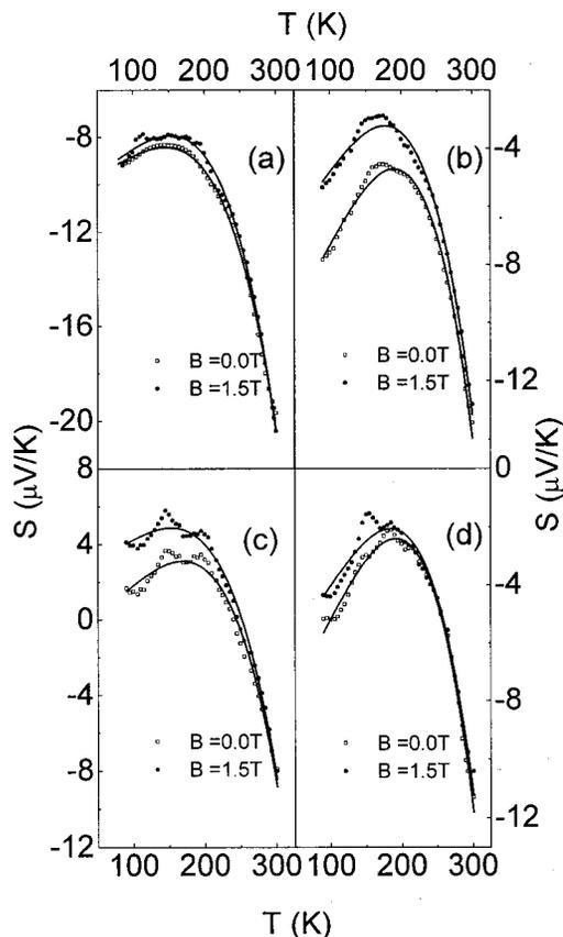
FIG. 9. Temperature and magnetic field ( $B=1.5$  T) dependent Seebeck coefficient ( $S$ ) of four different samples  $\text{La}_{0.7}\text{Ca}_{0.3-y}\text{Na}_y\text{MnO}_3$  with (a)  $y=0.05,$  (b)  $0.1,$  (c)  $0.15,$  and (d)  $0.3$ . Solid lines are best fit lines to Eq. (3).
