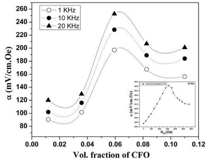
FIG. 4. Variation of the estimated  $\alpha_{\max}$  with CFO volume contents at various frequencies of the applied ac magnetic field. The inset shows the variation of the magnetoelectric coupling coefficient of 94.06 PLT15-5.94 CFO composite film with the dc bias magnetic field (measured at 20 kHz).
