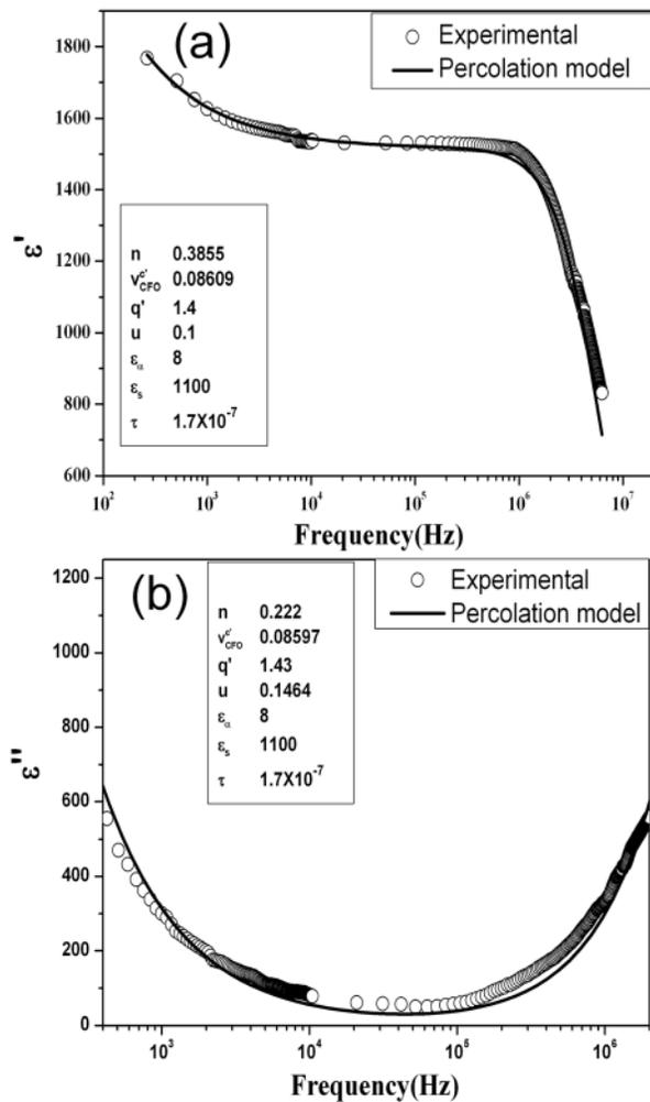
FIG. 3. Frequency dispersion of (a) the real and (b) imaginary part of dielectric constant of 0.92  $\text{Pb}_{0.85}\text{La}_{0.15}\text{TiO}_3$ -0.08  $\text{CoFe}_2\text{O}_4$  composite thin film. The symbols represent the experimental data and the solid lines are the non-linear best fit based on Eq. (4) for real, and Eq. (5) for imaginary part of the dielectric constant. The relevant best fitted parameters are indicated in the inset of the respective figures.
