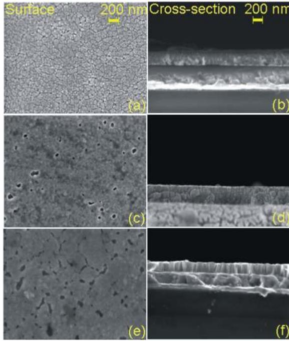
FIG. 1. (Color online) (a) Surface and (b) cross sectional morphology of  $\text{Pb}_{0.85}\text{La}_{0.15}\text{TiO}_3$ , (c) surface and (d) cross sectional surface morphology of  $0.92 \text{Pb}_{0.85}\text{La}_{0.15}\text{TiO}_3-0.08 \text{CoFe}_2\text{O}_4$  and (e) surface and (f) cross sectional surface morphology of  $0.88 \text{Pb}_{0.85}\text{La}_{0.15}\text{TiO}_3-0.12 \text{CoFe}_2\text{O}_4$  thin films.
