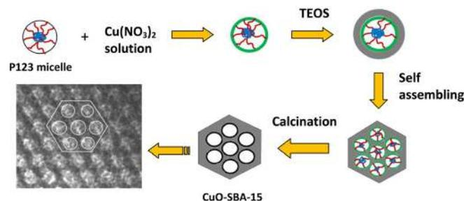
FIG. 1. Schematic representation of preparation of the CuO-SBA-15 nanocomposite.
