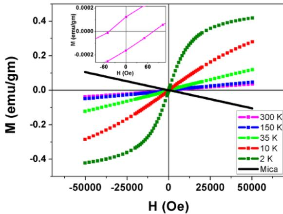
FIG. 4. Magnetization vs magnetic field at different temperatures (2, 10, 35, 150, and 300 K). (Inset) An enlarged view of the  $M$ - $H$  curve over the low field region at 300 K.
