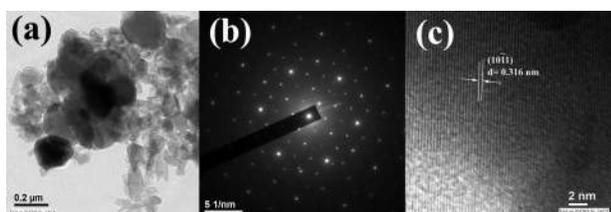
FIG. 2. (a) Transmission electron micrograph of CdS nanosheets. (b) Selected area electron diffraction pattern of nanosheets. (c) High resolution lattice image of a portion of CdS nanosheets.
