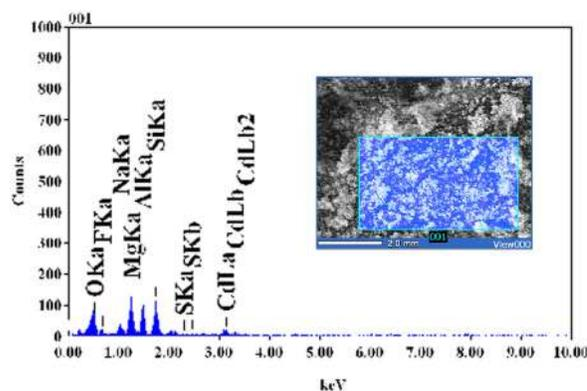
FIG. 3. EDAX analysis of CdS-mica nanocomposite.
