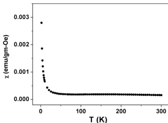
FIG. 5. Variation in magnetic susceptibility ( $\chi$ ) as a function of temperature for the CdS-mica nanocomposite under a magnetic field of 100 Oe in the zero field cooled condition.
