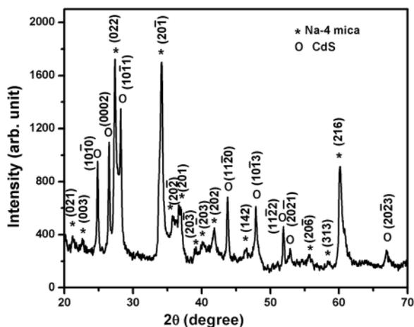
FIG. 1. X-ray diffractogram of CdS-mica nanocomposite. The Na-4 mica and CdS phases are marked with stars (\*) and open circles, respectively.
