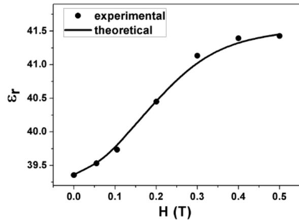
FIG. 6. Variation of dielectric constant with magnetic field for the CdS-mica nanocomposite at room temperature.
