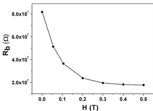
FIG. 7. Variation of resistance (extracted from analysis) of the CdS layer with magnetic field.
