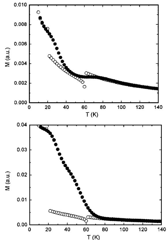
FIG. 4. Results of our simulations for a system in which the sample was cooled (open circle) at a magnetic field,  $H$ . At  $T=60$  K the field is switched off and the temperature of the system is arrested before restore the field  $H$  and at 20 K a field of  $2H$  (top panel) or  $5H$  (bottom panel) is applied. Note that the application of a large field erases the effect of the previous magnetic field switching off. The solid circles in the figure are the magnetization during heating cycle.
