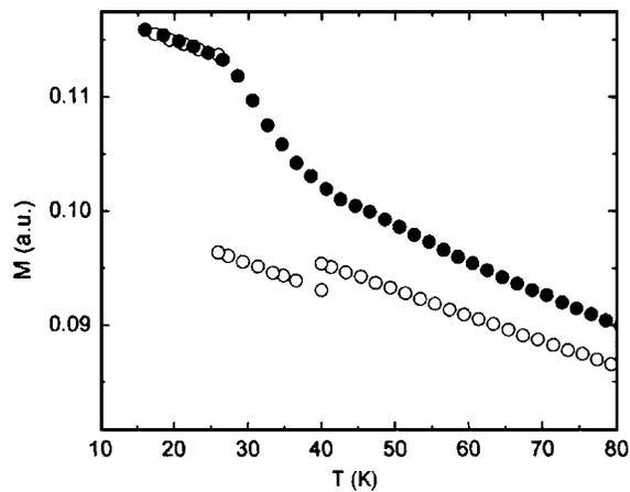
FIG. 3.  $M(T)$  curves for the cooling (open circle) and heating cycle (solid circle) while switching off the field at 40 K and applying an 800 Oe field at 24 K. In this case, the signature of the field switching off at 40 K is erased from the heating curve.
