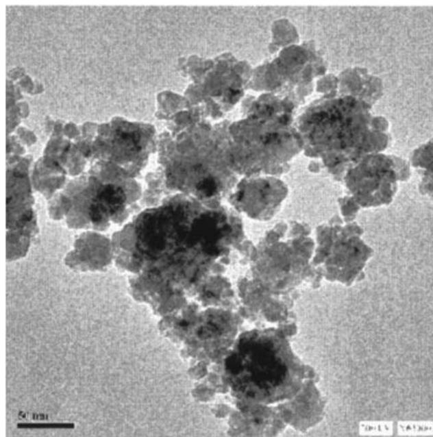
FIG. 1. TEM micrographs of  $\text{Ni}_{0.35}\text{Zn}_{0.65}\text{Fe}_2\text{O}_4$  particles with diameters ranging from 10 to 100 nm.
