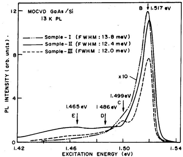
FIG. 2. PL spectra for GaAs/Si samples grown under three different conditions.
