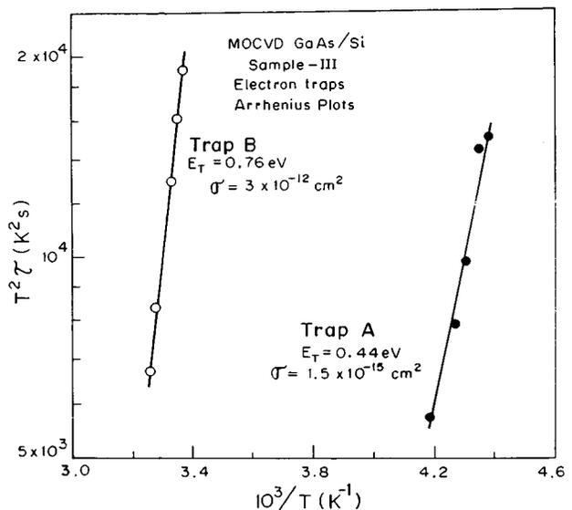
FIG. 5. Arrhenius plots for electron traps A and B, measured from the DLTS data of sample III.
