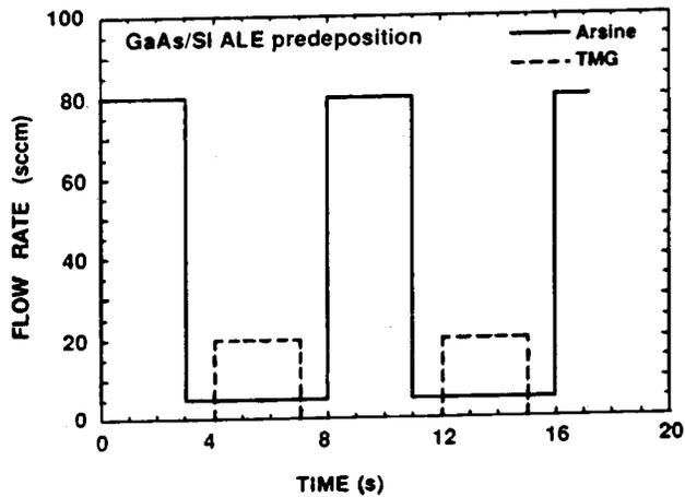
FIG. 1. Flow modulation scheme for ALE growth of predeposition layer in GaAs/Si.
