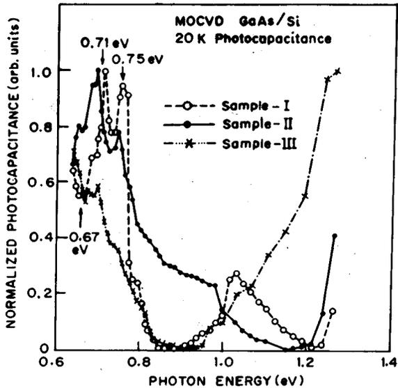
FIG. 6. Photocapacitance spectra of electron and hole traps in samples I, II, and III.
