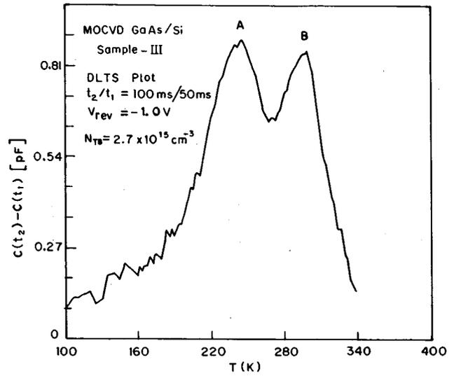
FIG. 4. DLTS spectrum of electron traps in sample III. The trap concentration shown here corresponds to that of trap B which almost equals the concentration of trap A.
