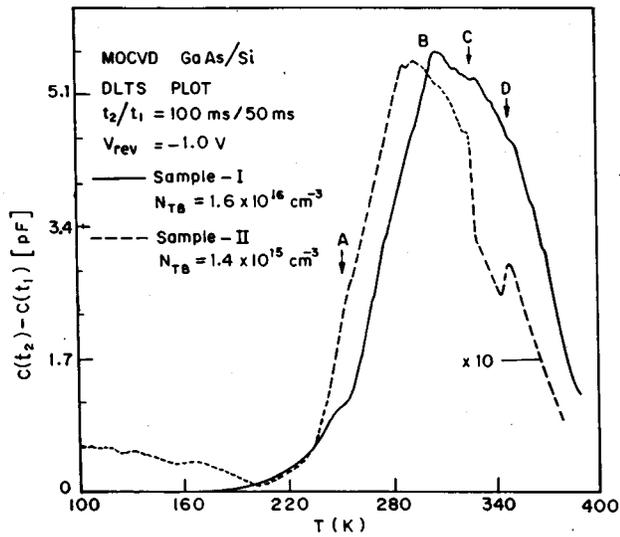
FIG. 3. DLTS spectra of electron traps in sample I and II, indicating concentration of trap B only.
