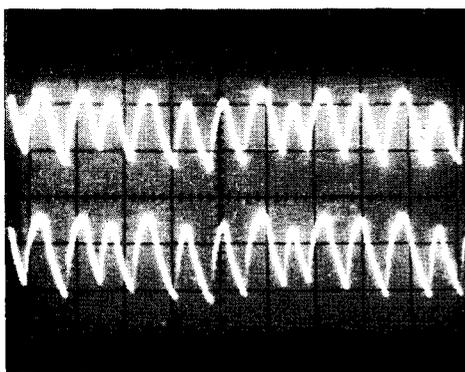
FIG. 2. An example of the oscillations at two azimuthal probes separated by  $90^\circ$  (sweep speed 0.5 msec/cm), the pattern being same for other azimuthal separations. All the probes are kept at a radial location  $r \approx 1$  cm.
