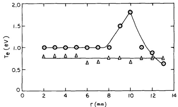
FIG. 5. Radial electron temperature ( $T_e$ ) distributions:  $\odot$  for grids floating and  $\triangle$  for grids connected to anodes, the discharge conditions being the same as Fig. 3.
