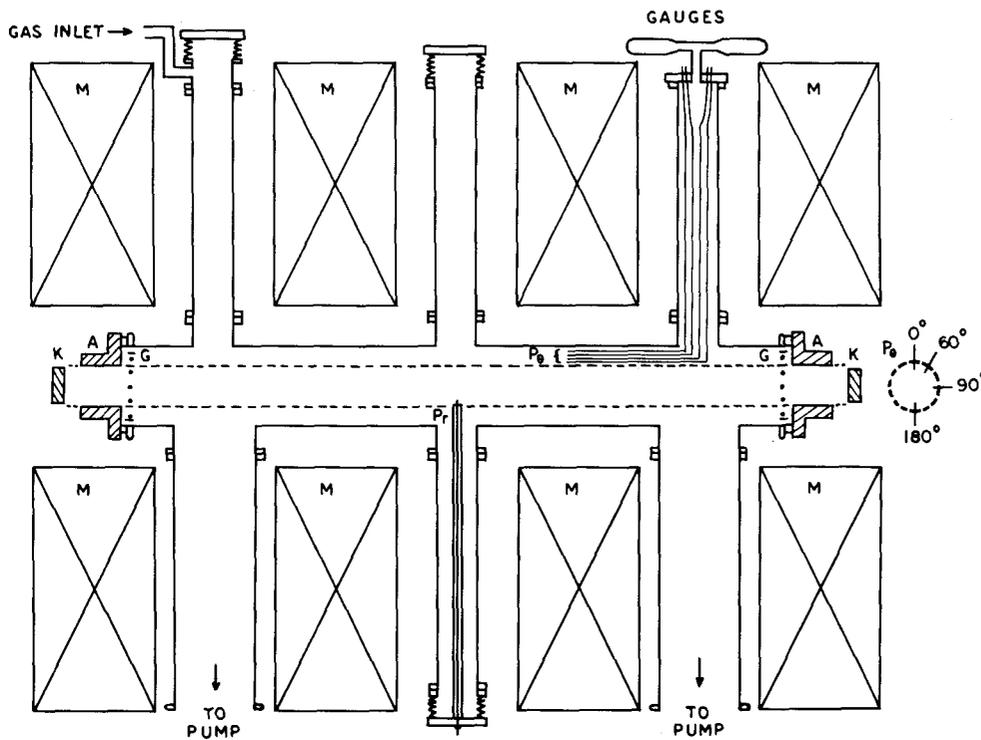
FIG. 1. Schematic diagram of the experimental arrangement;  $P_r$ : radially movable Langmuir probe;  $P_\theta$ : azimuthal probe assembly; M: magnet coils; dotted horizontal lines: the plasma boundary.
