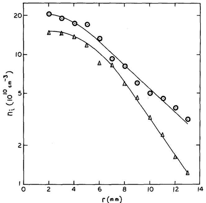
FIG. 3. Radial ion density ( $n_i$ ) distributions for nitrogen:  $\odot$  for grids floating and  $\triangle$  for grids connected to anodes.  $r$  denotes radial position of the probe. Gas pressure is  $3 \times 10^{-2}$  Torr; discharge current is 30 mA; and magnetic field is 280 G.
