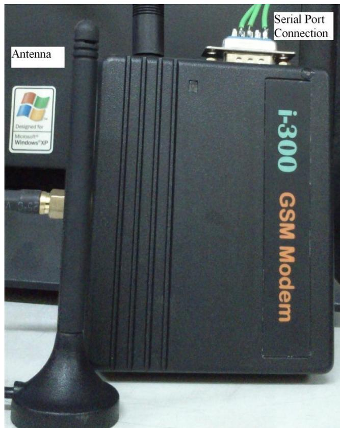
Figure 7. An 'i-300' GSM modem.
