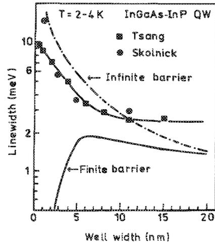
FIG. 1. Variation of photoluminescence linewidth with the thickness of the quantum well. Squares and circles: experimental data obtained by Tsang (Ref. 8) and Skolnick *et al.* (Ref. 9), respectively. Dash dotted curve: values obtained from Eq. (8). Solid curve: values of LW taking leakage of wave function into account.
