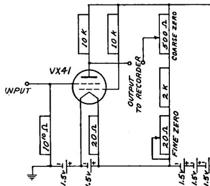
FIG. 1. Circuit diagram of the recorder for use with the Brown Instrument Company's "Elektronik" recorder.
