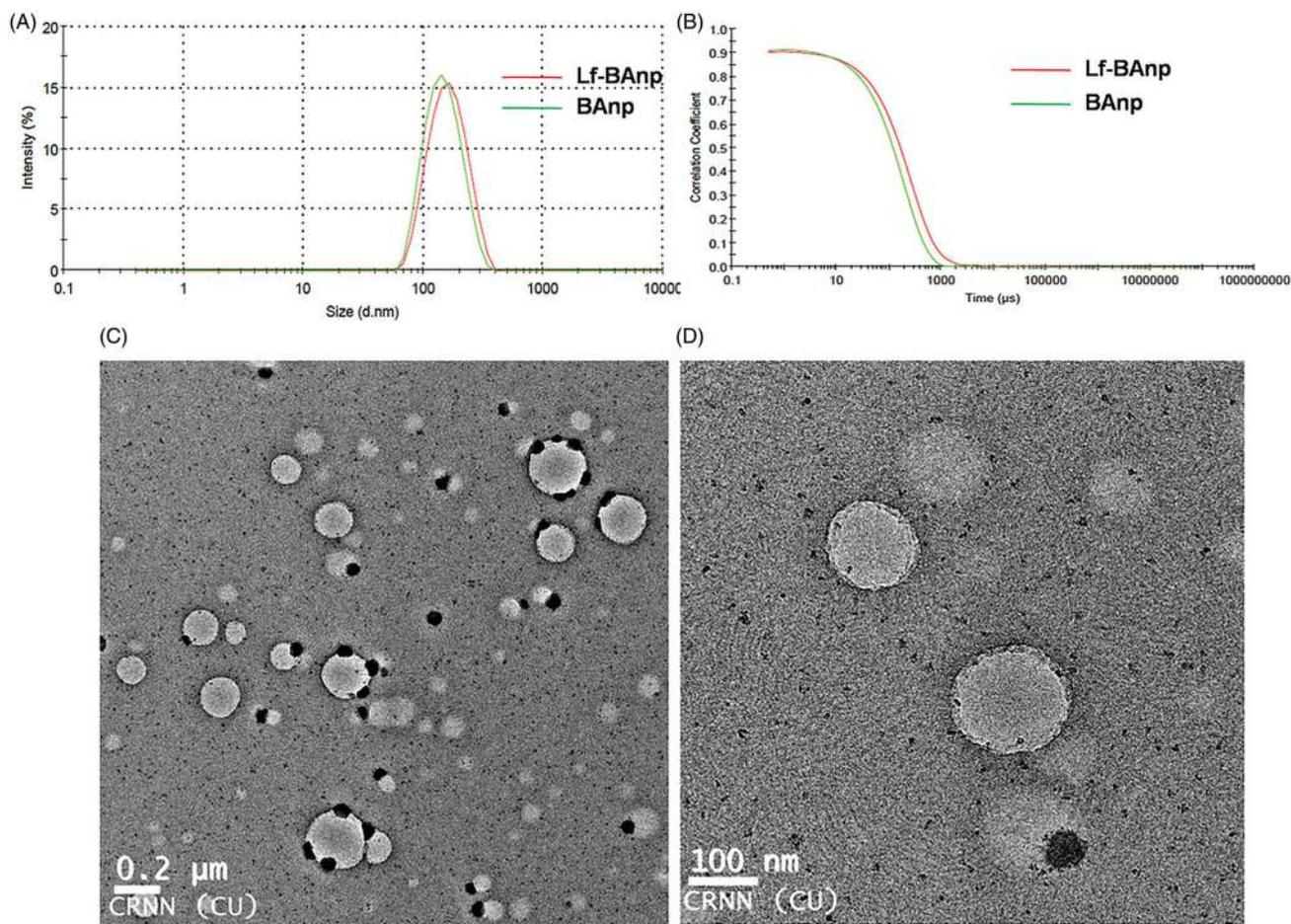
**Figure 1.** (A) Particle size distribution in scattering intensity measured in DLS and (B) corelogram overlay of Lf-BAnp and BAnp dispersed in aqueous medium. (C) HR-TEM study of Lf-BAnps and (D) High magnification image of that nanoparticle.
