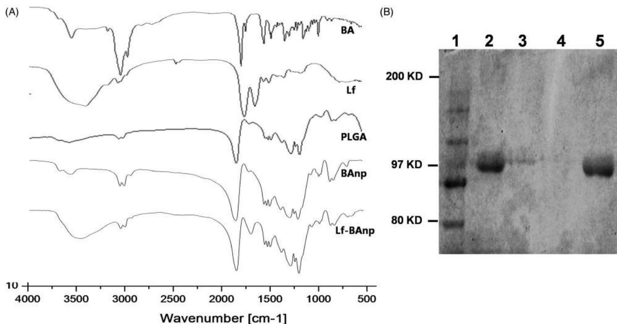
**Figure 2.** (A) FT-IR spectra of BA, Lf, PLGA, BAnp and Lf-BAnp, scanned over a range of 4000 to 400  $\text{cm}^{-1}$  and (B) SDS-PAGE studies of nanoparticles. Lanes: 1. Marker, 2. Lf-BAnp, 3. BAnp and Lf physical mixture, 4. BAnp and 5. Lf.
