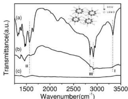
FIG. 1. Shows the FTIR spectrum of pure ODA, LSMO-ODA, and uncoated LSMO powders as shown in (a), (b), and (c), respectively, recorded with a KBr pellet. The inset shows the schematic of the type of electrostatic interaction and probable microscopic structure of the LSMO sample being encapsulated with ODA molecules.
