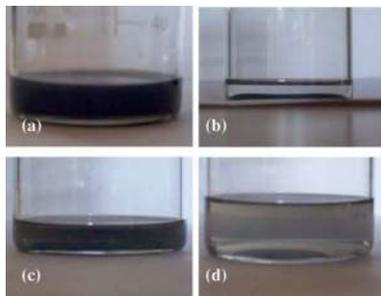
FIG. 4. (a) shows the decanted solution prior to purification, showing uniform suspension of ODA coated LSMO particles. (b) shows the particles precipitated out of methanol after two washing cycles. (c) and (d) show the results after refluidization in chloroform of the dry ODA coated powder at two different concentrations, namely, 0.1 and 0.05 mg/ml, respectively, clearly indicating fully uniform dispersion once again.
