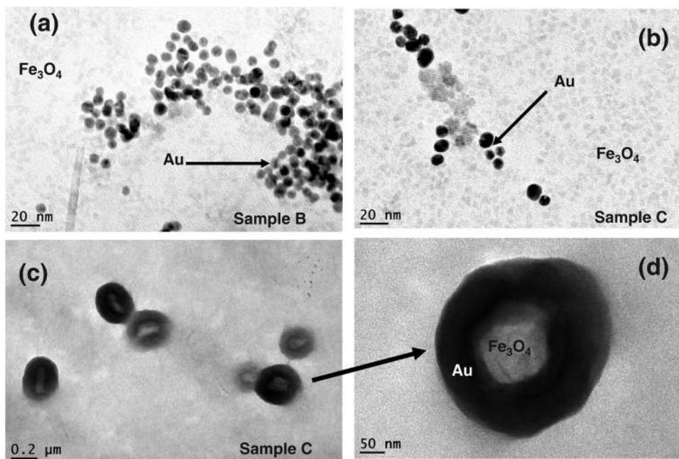
FIG. 1. (See online for better contrast of  $\text{Fe}_3\text{O}_4$  particles.) Transmission electron micrographs of the (a) Sample B (Low-Au) and (b–d) Sample C (High-Au) nanocomposites.  $\text{Fe}_3\text{O}_4$  can be seen in the background as faint particles of size 3–4 nm. Au particles are darker and are marked by arrows. Core( $\text{Fe}_3\text{O}_4$ )-shell(Au) structures seen in Sample C are shown in (c) and (d).
