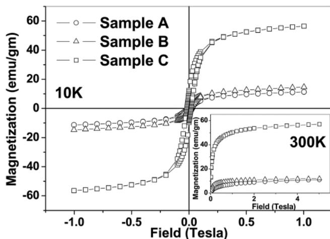
FIG. 3. Magnetization vs H for Sample A (Pure), Sample B (Low-Au), and Sample C (High-Au) taken at 10 K and inset: 300 K.
