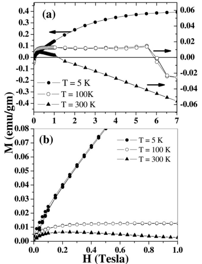
FIG. 6. (a) Magnetization vs  $H$  for the Au-citrate sample taken at  $5, 100,$  and  $300$  K up to a field of (a)  $7$  T and (b) expanded scale up to  $1$  T.
