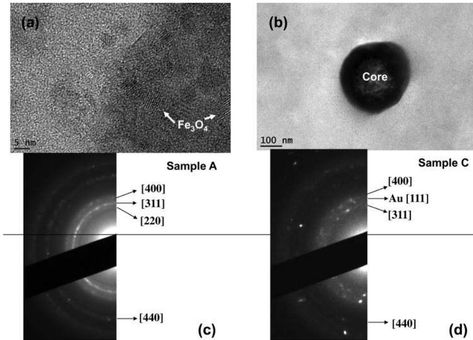
FIG. 2. Transmission electron micrographs and electron diffraction: (a) and (c) Sample A (Fe<sub>3</sub>O<sub>4</sub>); (b) and (d) core of the Sample C core shell particles. The diffraction rings in the (d) clearly shows presence of Fe<sub>3</sub>O<sub>4</sub>.
