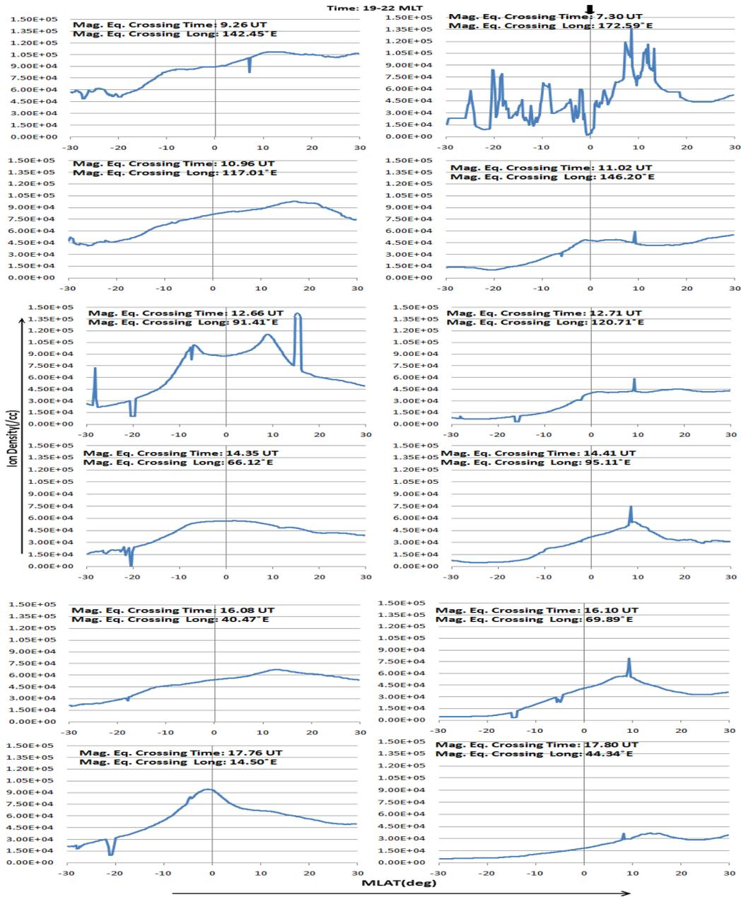
**Figure 4.** Total Ion Density ( $\text{cm}^{-3}$ ) variation as observed by the DMSP f12,f14 and f15 satellites on May 30, 2005 from morning to post-sunset UT. Presence of irregularity is indicated by black down arrow.
