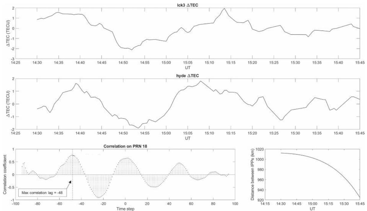
**Figure 8.** Time series of  $\Delta TEC_{VAR}$  from LCK3 (top) and HYDE (middle) between 14:30 UT and 15:45 UT on 8 September for PRN18. (bottom left) Corresponding cross-correlation coefficient between -45 and +45 min corresponding to -90 and 90  $\Delta TEC$  timestep (30 s), respectively. (bottom right) distance between IPP of PRN18 as seen from LCK3 and HYDE as a function of time.
