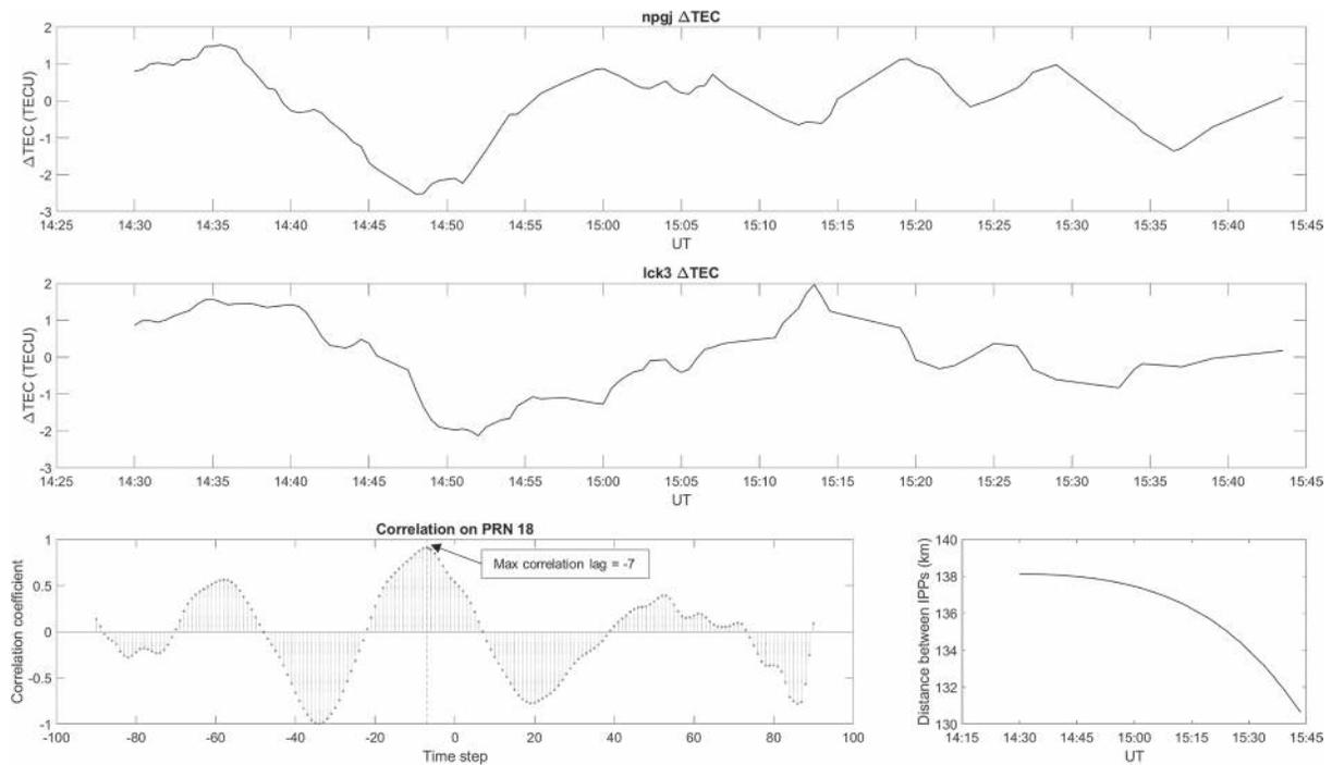
**Figure 7.** Time series of  $\Delta TEC_{VAR}$  from NPGJ (top) and LCK3 (middle) between 14:30 UT and 15:45 UT on 8 September for PRN18. (bottom left) Corresponding cross-correlation coefficient between -45 and +45 min corresponding to -90 and 90  $\Delta TEC$  timestep (30 s), respectively. (bottom right) distance between IPP of PRN18 as seen from NPGJ and LCK3 as a function of time.
