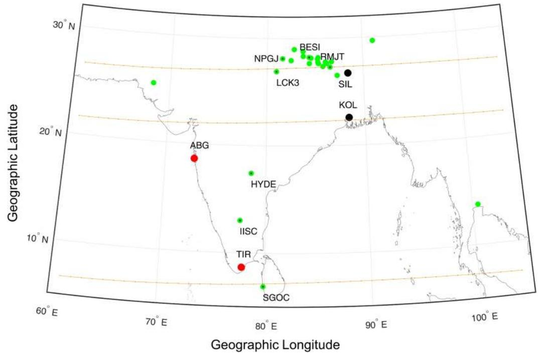
**Figure 2.** Network of the stations providing the data. Red dots: magnetometers; black dots: scintillations monitors; green dots: GPS stations. In green dots with a black dot inside, a subset of GPS stations used for TIDs detection and ROTI time profiles (see Figure 4). The orange lines represent the position of the dip equator and the isoclinic lines at +15°N and +20°N.
