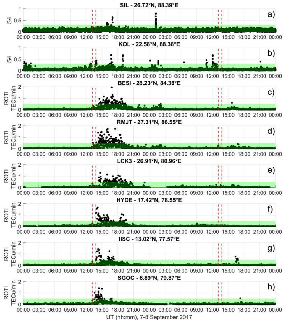
**Figure 4.** Time profiles of S4 (a–b) and of ROTI (c–h) obtained by considering all satellite in view from the station indicated in each panel during seven and 8 September. The red-dashed lines indicate the time of the passage of the Sun terminator at the station location and at an altitude of 120 km and of 350 km. The green shaded area indicates the ranges  $S4 < 0.3$  and  $ROTI < 0.5$  TECu/min.
