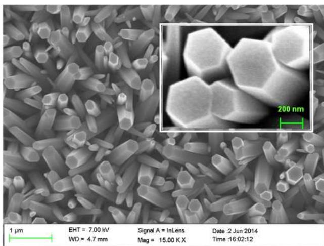
FIG. 1. The FESEM image of the grown ZnO-nanowires on p-Si substrate. Image in the inset shows the ZnO hexagonal structures.
