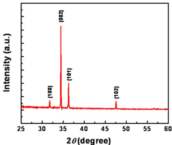
FIG. 2. Plot of the XRD pattern of ZnO nanowires. The dominant peak appearing from [002] orientation indicates the growth along c-axis or (001) direction.
