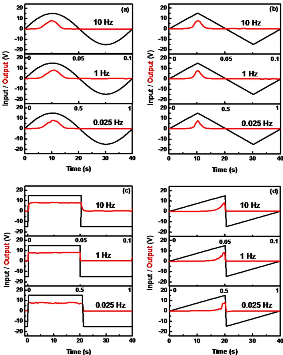
FIG. 5. Plots of output responses of the single n-ZnO-nanowire/p-Si diode in response to the standard pulses: (a) sinusoidal, (b) triangular, (c) square, and (d) saw-tooth at different frequencies.
