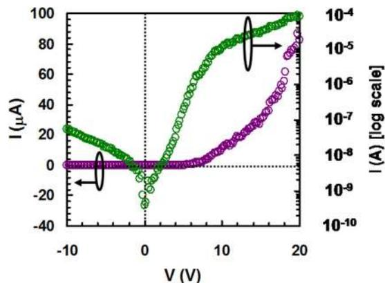
FIG. 4. Plots of the current-voltage characteristics of a single n-ZnO-nanowire/p-Si junction diode.
