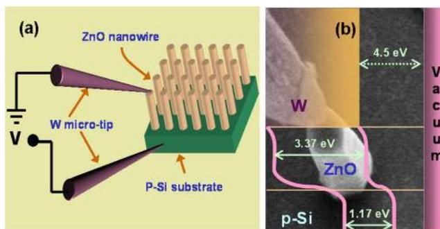
FIG. 3. (a). Schematics of the electrical measurement set up; (b) FESEM image of the tungsten (W) probe-tip in contact with a single standalone ZnO-nanowire on p-Si substrate during the measurement. The corresponding schematic band alignment across the junction is also overlapped on the structure.
