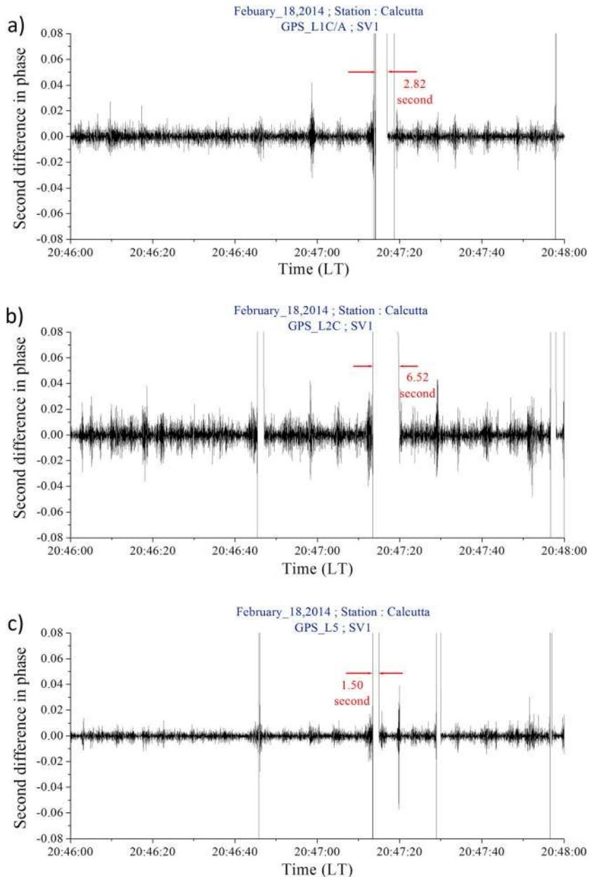
**Figure 5.** Case study of cycle slips observed on same SV link around same time interval at triple frequency of GPS on 18 February 2014. (a) Second difference in phase (cycles) at L1 C/A on SV1 during 20:46–20:48 LT. (b) Second difference in phase (cycles) at L2C on SV1 during 20:46–20:48 LT. (c) Second difference in phase (cycles) at L5 on SV1 during 20:46–20:48 LT. GPS = Global Positioning System.
