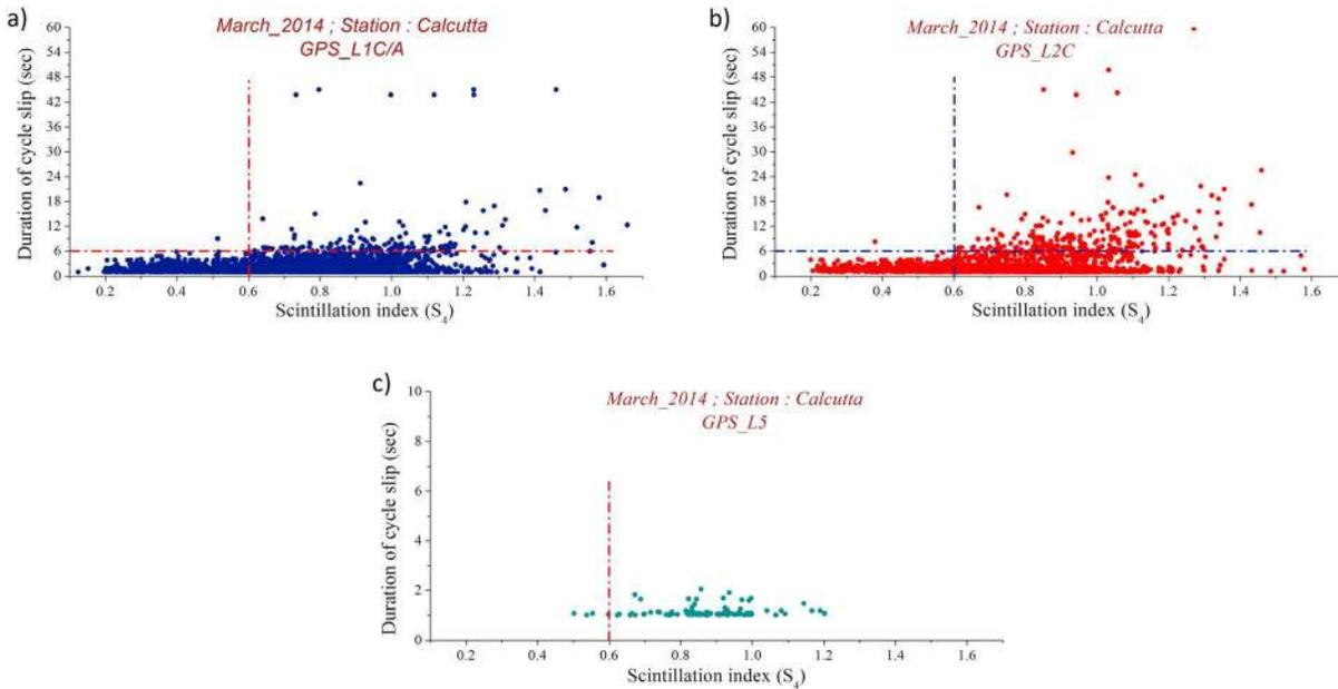
**Figure 3.** A correlation between intensity of amplitude scintillation index ( $S_4$ ) and duration of cycle slips observed at (a) L1 C/A, (b) L2C, and (c) L5 of GPS during March 2014 from Calcutta. GPS = Global Positioning System.
