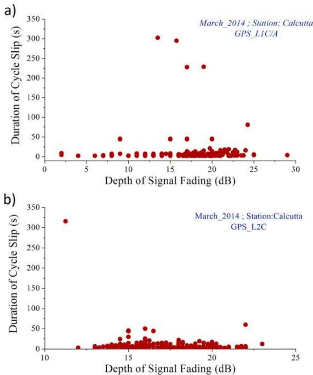
**Figure 4.** A relation between depths of signal fading and duration of cycle slip for March 2014 on all SVs at (a) GPS L1 C/A and (b) GPS L2C. GPS = Global Positioning System.
