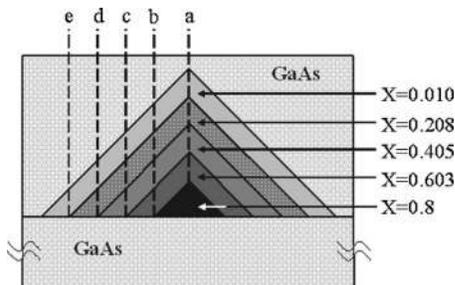
FIG. 3. Model of Fig. 2(b) showing the variation of indium which is assumed to be a linear gradient of five concentrations from the central core to the outer periphery.
