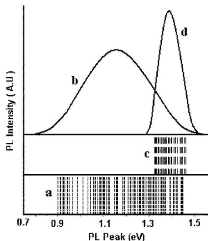
FIG. 4. Schematic diagram of the computed PL spectra for triangular and rectangular QWs corresponding to Tables I and II.
