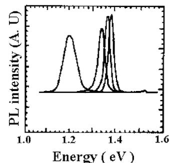
FIG. 1. Blueshifts in the PL from  $\text{In}_x\text{Ga}_{1-x}\text{As}/\text{GaAs}$  QDs on annealing.
