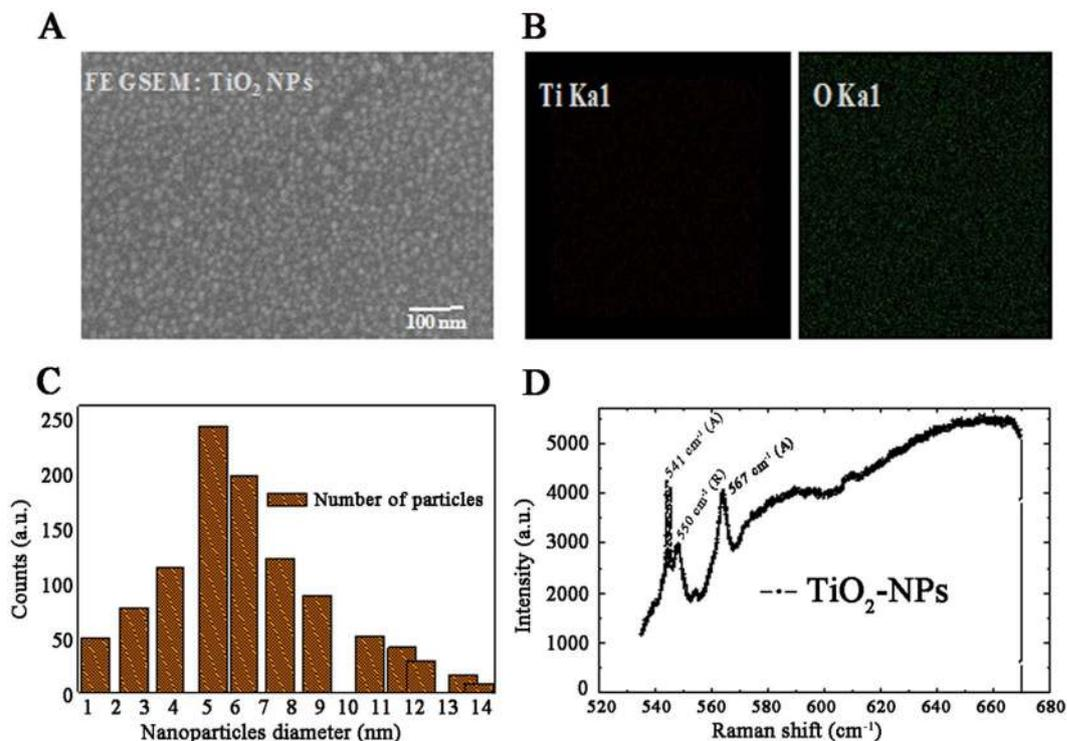
**Figure 1.** Structural behaviour of TiO<sub>2</sub>-NPs. (A) Top view FESEM images of nano-sized TiO<sub>2</sub> particles. (B) Element mapping of the sample. (C) Particle histogram of Image 1(A). (D) Raman spectrum of TiO<sub>2</sub>-NPs.
