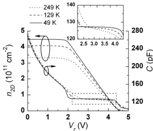
FIG. 4.  $n_{2D}$  and the simulated capacitance of the structure as a function of reverse bias  $V_r$  at different temperatures. The selected portion of the capacitance plots is enlarged in the inset.
