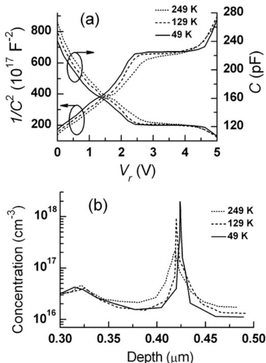
FIG. 1. Experimental results: (a)  $C$ - $V$  characteristics of the structure at different temperatures and (b) apparent carrier profiles at different temperatures.
