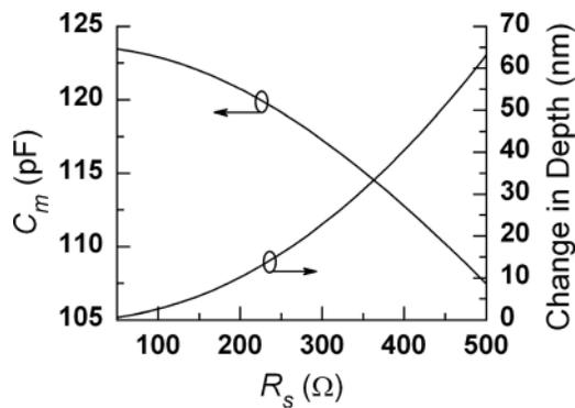
FIG. 5. The measured capacitance  $C_m$  and the change in the depth as a function of the series resistance  $R_s$ . The variation is shown with respect to the experimental peak capacitance at 249 K.
